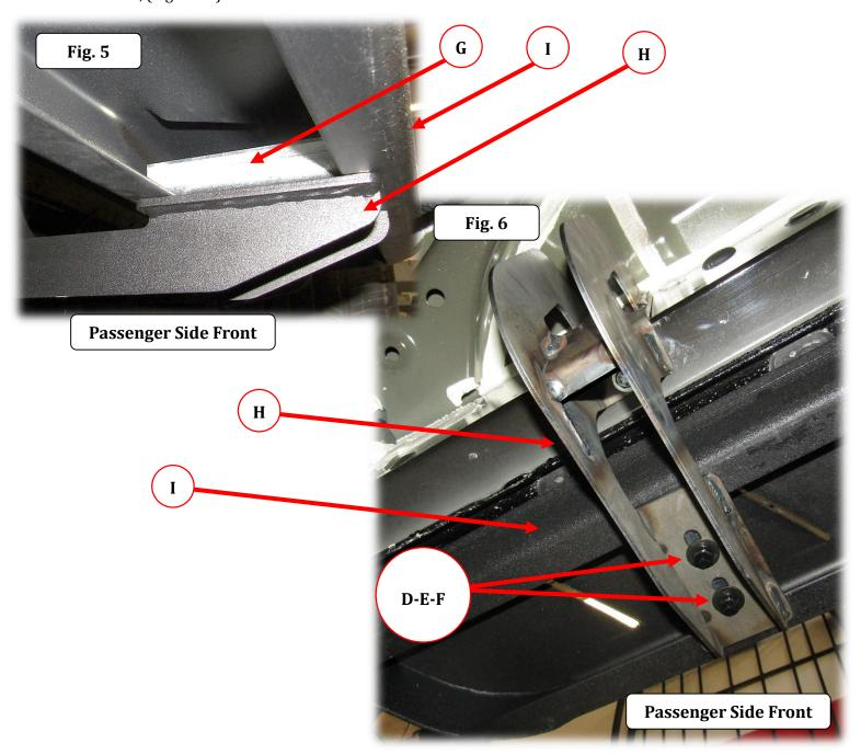
**Step-5** Align the running board with the vehicle and tighten all supplied nuts and bolts securing the running board and bracket assembly. Repeat to install the brackets and running board on the driver side of the vehicle.
