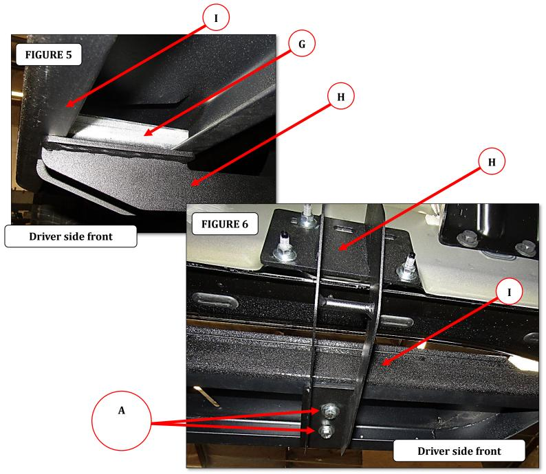
**Step-5** Align the running board with the vehicle and tighten all supplied nuts and bolts securing the running board and bracket assembly. Repeat to install the passenger running board. **Be sure to position the bar with the logo towards the rear**.
