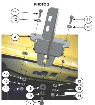
**STEP 3.** REPEAT THE ABOVE PROCEDURE TO INSTALL (1) MIDDLE MOUNTING BRACKETS AT THE CENTER POSITION. DO NOT TIGHTEN. **PHOTO** #3 & **PHOTO** #4
