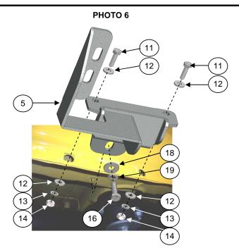
**STEP 6.** PLACE THE U BRACKET INSIDE RB10 SIDE STEP, PLACE THE RB10 SIDE STEP ON BRACKETS AND ATTACH WITH: 5/16" HEX HEAD BOLT, 5/16" FLAT AND LOCK WASHER (BLACK PLATED), BY EACH BRACKET. **PHOTO #7**
