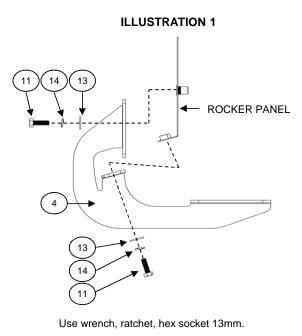
Step-2 Locate in the center and rear in the rocker panel of the vehicle the hole and insert a M8 clip nut. SEE PICTURE 3 & 4 & 5. Place the bracket and attach with: M8 hex head bolt, M8 flat and lock washers, M8 hex nut (zinc plated), according to the ILLUSTRATION 2. Leave loose. Repeat for the opposite side.
