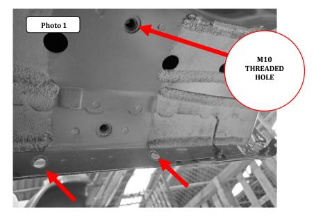
**Step-2** Attach the driver side Front bracket to the pinch mold using (2) 1/4" x 1" hex head bolts, (4) 1/4" flat washers, (2) 1/4" lock washers and (2) 1/4" hex nuts, and to the underside of the body using (1) M10 x 25mm hex bolt, (1) M10 lock washer and (1) M10 flat washer. **Photo 2 & 3.** Leave the nuts and bolts loose for final adjustment.
