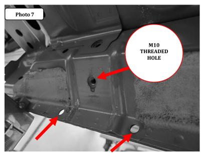
**Step-6 (Four Door Models Only)** Attach the driver side Rear bracket to the pinch mold using (2) 1/4" x 1" hex head bolts, (4) 1/4" flat washers, (2) 1/4" lock washers and (2) 1/4" hex nuts, and to the underside of the body using (1) M10 x 25mm hex bolt, (1) M10 lock washer and (1) M10 flat washer. **Photo 8 & 9.** Leave the nuts and bolts loose for final adjustment.
