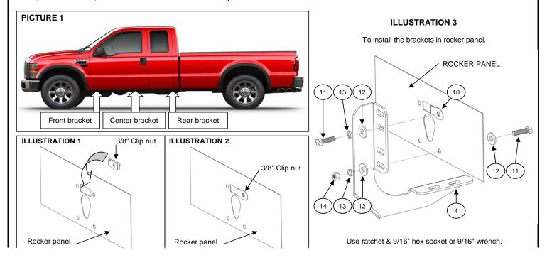
**Step-3** Place the U bracket and attach with: 5/16" hex head bolt, 5/16" Flat and lock washer (black plated), by each bracket. **SEE ILLUSTRATION 4 & 5.** Repeat for the opposite side. Leave loose.
