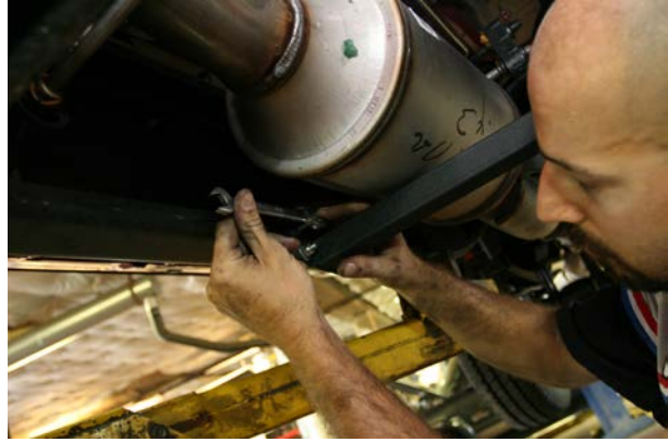
(Fig. 8) Tighten cross member against frame using 5/16" plated bolts, washers and nylon locking nuts provided. Note exhaust particulate filter above cross member.
