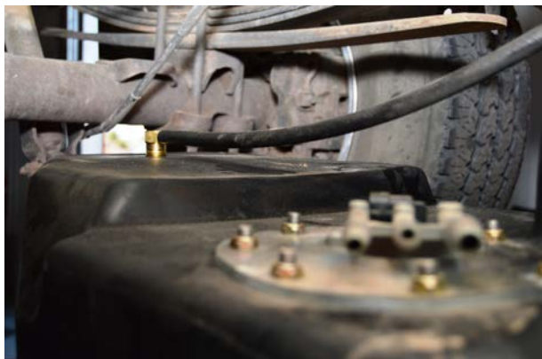
(Fig. 5) Rear rollover valve with vent hose attached.
