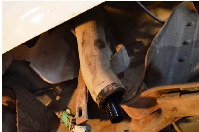
(Fig. 10) On vehicles with LB7 engines only, an interior fill hose is located inside the main fill hose. The tank vents through the space provided between the two hoses. Ten (10) inches needs to be cut off of the interior hose on end that goes to the tank as shown.
