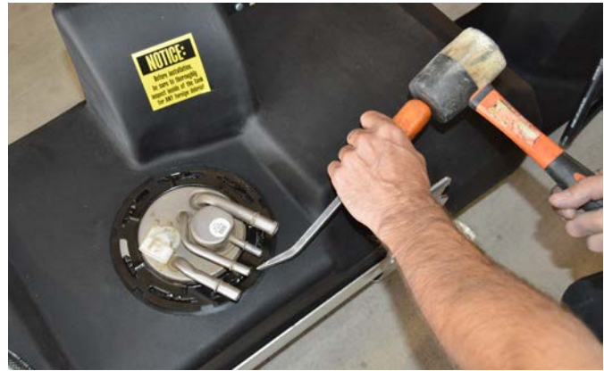
(Fig. 4) Tighten the original equipment hold-down ring by turning it clockwise as far as it will go.
