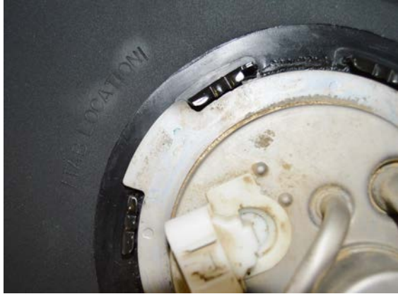
(Fig. 3) Make sure the sending unit tab lines up with the "tab location" mark.
