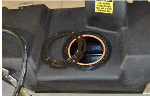
(Fig. 2) TITAN sending unit mount before sending unit is installed. Reuse the Top Locking Ring from the OEM tank.
