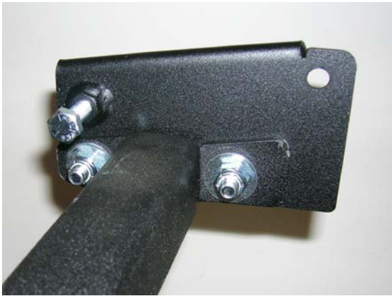
(Fig.9) Shown: Right-Hand Bracket for GM Cross Bar. The Cross Bar is held fast by tightening the 5/16" cap screw seen here at the upper left hand corner of the bracket. It is recommended that the installer position the Cross Bar, tighten down the cap screw as shown, and then drill a hole in the frame lip through the hole seen in the right-hand corner of the bracket. A 5/16" cap screw and nylon locking nut are provided for fastening this hole. It is advisable to apply Loctite Thread locker or equivalent to the bolts.
