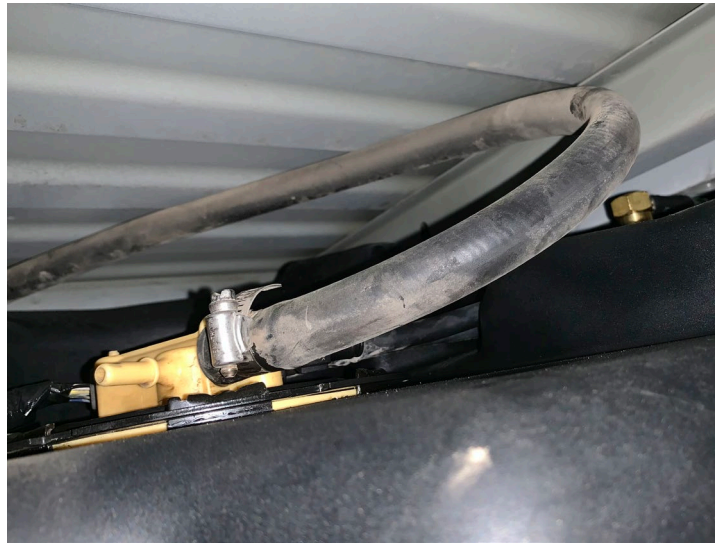
(Fig. 7) Lift tank high enough to reconnect electrical cable and vent hose to sending unit.
