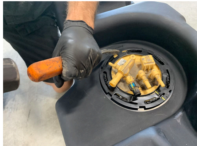
(Fig. 5) Tighten the top TITAN Torque hold-down ring onto the sending unit by turning it clockwise as far as it will go.
