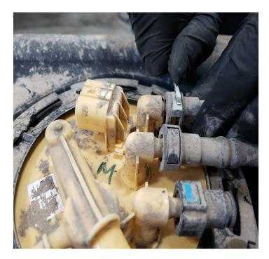
Use a mallet and screwdriver or punch to loosen the OEM hold-down ring on the sending unit by tapping it and turning it counter-clockwise.
