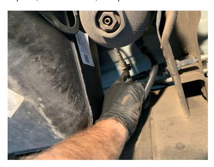
Loosen and remove OE tank straps by undoing the bolts at outside of tank, then unhook straps on the inside to lower tank a few inches.
