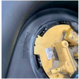
Place the included TITAN Torque Ring, top hold-down ring onto the lugs and the sending unit and turn it clockwise as far as it will go (see Fig. 5).
