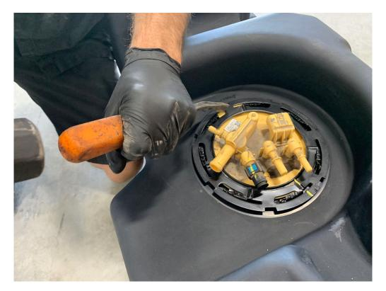
17 Retrieve the fuel lines from the OE tank and attach the suction and return fuel lines to the sending unit which is now installed in the replacement tank. After attaching them to the sending unit, lay the fuel lines into the fuel line groove provided in the top of the replacement tank. If desired, it is good practice to tie the two lines together with snap ties.
