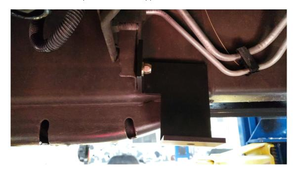
21 Place the tank on a transmission jack. Then lift the tank high enough to reconnect the sending unit electrical connection and the vent hose to the sending unit.
