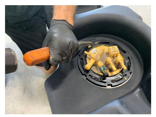
17 Retrieve the fuel lines from the OE tank and attach the suction and return fuel lines to the sending unit which is now installed in the replacement tank. After attaching them to the sending unit, lay the fuel lines into the fuel line groove provided in the top of the replacement tank.
