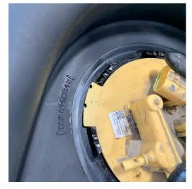
Place the top hold-down ring onto the lugs and the sending unit and turn it clockwise as far as it will go (see Fig. 5).
