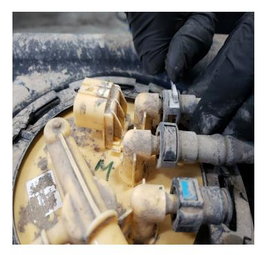
Use a mallet and screwdriver or punch to loosen the OEM hold-down ring on the sending unit by tapping it and turning it counter-clockwise. Remove the sending unit from the OE tank. Do NOT reuse factory O-ring seal.
