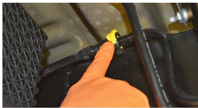
(Fig. 6) Fuel line coupler located on the frame in front of the water separator.
