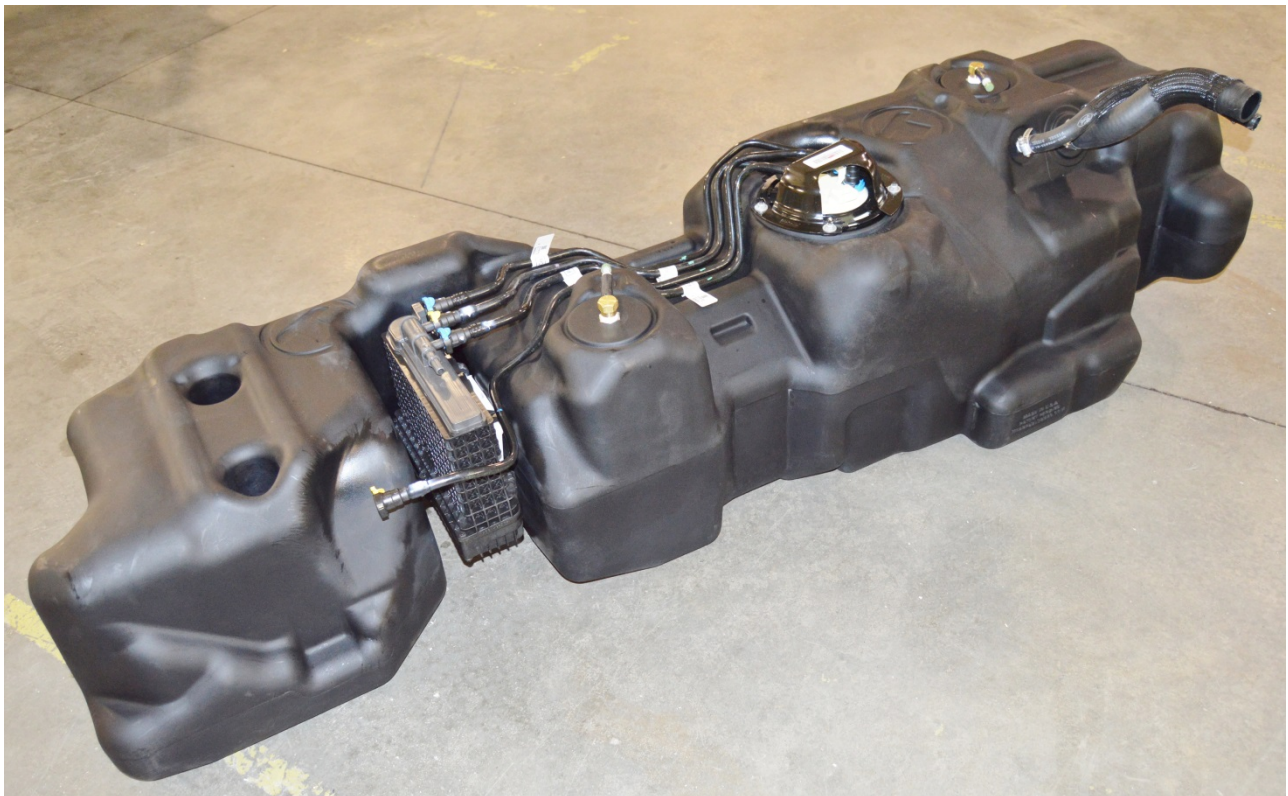
(Fig. 14) TITAN 7020217 tank shown with sending unit, water separator, fuel lines, sending unit guard, and fill and vent hoses installed; ready for installation into the vehicle.
