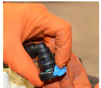
(Fig. 7): Method for Disconnecting Fuel Line Couplings: The majority of the couplings involved in this installation are of the quick connect type shown in left photo above. To disconnect, a) Slide the tab that has teeth on its edge outwards as shown in the center photo. b) Next, press the rounded button, as shown in the right photo, and pull the coupling apart. The coupling shown in Fig. 5 functions differently, see Step no. 9 for it.
