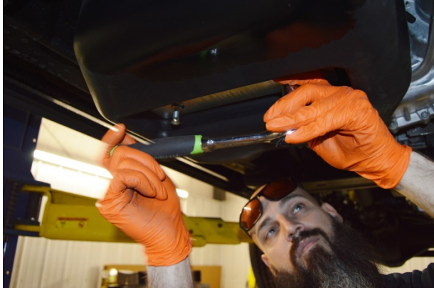
(Fig. 16) Tighten Front Support Assembly to 15 lb.-ft.
