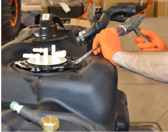
(Fig. 12) Reuse the OEM hold-down ring to mount the sending unit in the TITAN tank. Tighten by turning it clockwise as far as it will go.
