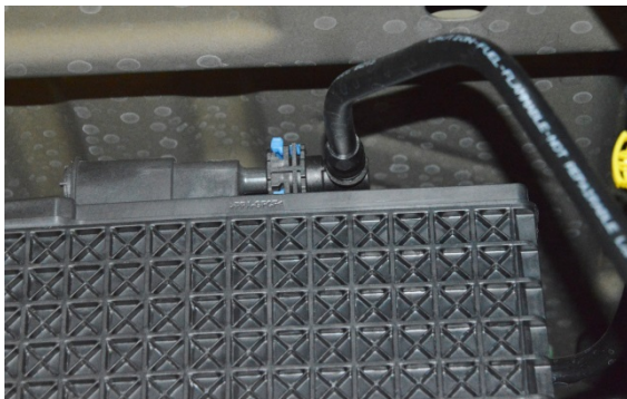
(Fig. 5) Fuel line connector at top of the separator.
