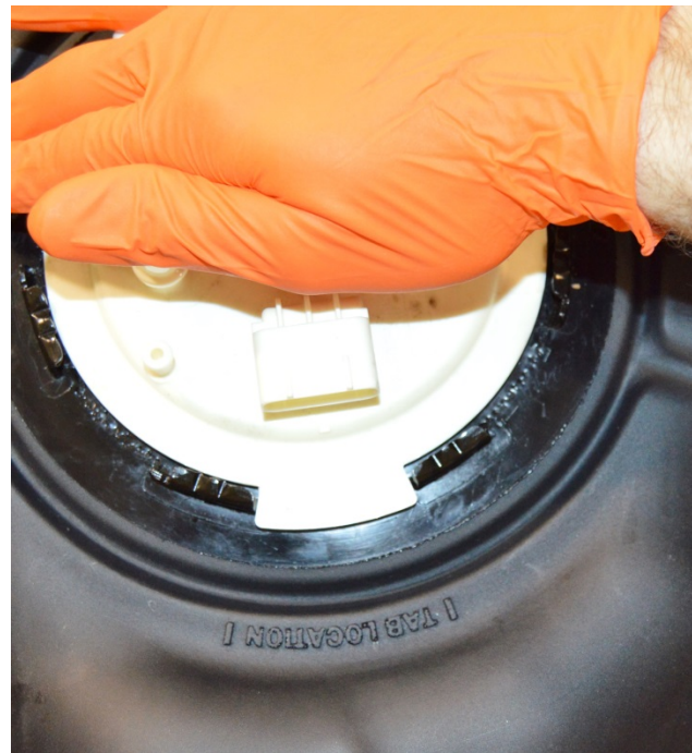
(Fig. 11) Line the tab on the sending unit up with the "tab location" mark on the TITAN tank.
