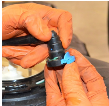
(Fig. 7): Method for Disconnecting Fuel Line Couplings: The majority of the couplings involved in this installation are of the quick connect type shown in left photo above. To disconnect, a) Slide the tab that has teeth on its edge outwards as shown in the center photo. b) Next, press the rounded button, as shown in the right photo, and pull the coupling apart. The coupling shown in Fig. 5 functions differently, see Step no. 9 for it.
