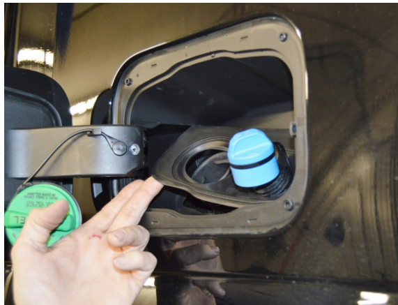
(Fig. 1) Loosen and remove rubber seal.
