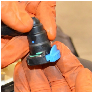
(Fig. 7): Method for Disconnecting Fuel Line Couplings: The majority of the couplings involved in this installation are of the quick connect type shown in left photo above. To disconnect, a) Slide the tab that has teeth on its edge outwards as shown in the center photo. b) Next, press the rounded button, as shown in the right photo, and pull the coupling apart. The coupling shown in Fig. 5 functions differently, see Step no. 9 for it.
