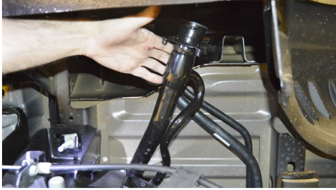
(Fig. 3) Move fill spout assembly toward vehicle frame to gain access to the hose clamps.
