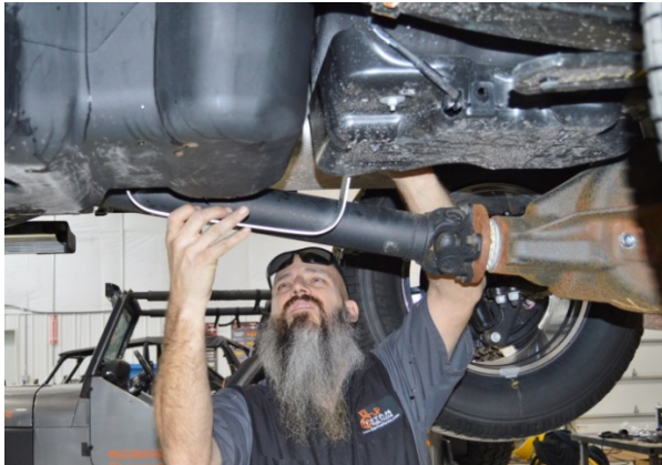
(Fig. 13) To install the new straps, turn and hook on inboard side of the tank, then rotate. Then tighten bolts on the outboard side.
