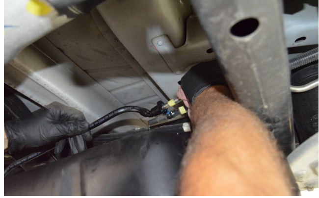
(Fig. 12) Connect fuel line couplings at the front of the tank before it is lifted all the way into place.
