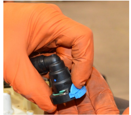
(Fig. 3): Method for Disconnecting Fuel Line Couplings: The couplings involved in this installation are of the quick connect type shown in left photo above. To disconnect, a) Slide the tab that has teeth on its edge outwards as shown in the center photo. b) Next, press the rounded button, as shown in the right photo, and pull the coupling apart.
