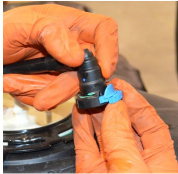
(Fig. 3): Method for Disconnecting Fuel Line Couplings: The couplings involved in this installation are of the quick connect type shown in left photo above. To disconnect, a) Slide the tab that has teeth on its edge outwards as shown in the center photo. b) Next, press the rounded button, as shown in the right photo, and pull the coupling apart.
