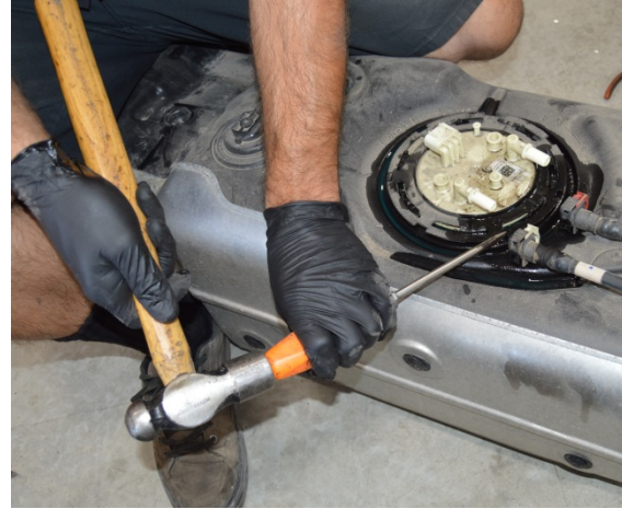
(Fig. 5) Loosen the OEM hold-down ring by turning it counter-clockwise.
