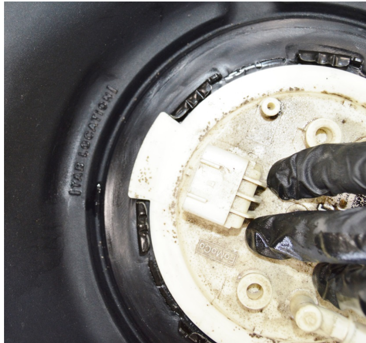
(Fig. 7) Line the tab on the sending unit up with the tab location marks on the TITAN tank.
