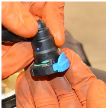
(Fig. 3): Method for Disconnecting Fuel Line Couplings: The couplings involved in this installation are of the quick connect type shown in left photo above. To disconnect, a) Slide the tab that has teeth on its edge outwards as shown in the center photo. b) Next, press the rounded button, as shown in the right photo, and pull the coupling apart.
