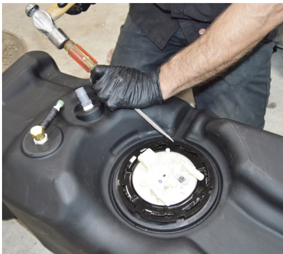
(Fig. 9) Use the OEM hold-down ring and tighten it by turning it clockwise as far as it will go.
