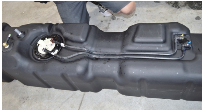
(Fig. 10) Fuel lines installed on the new TITAN tank.
