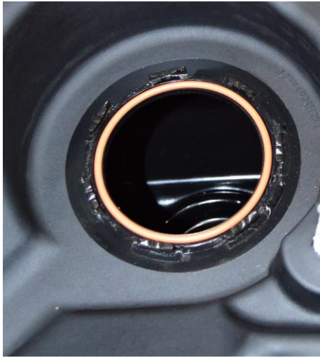
(Fig. 3) O-Ring gasket shown installed correctly.
