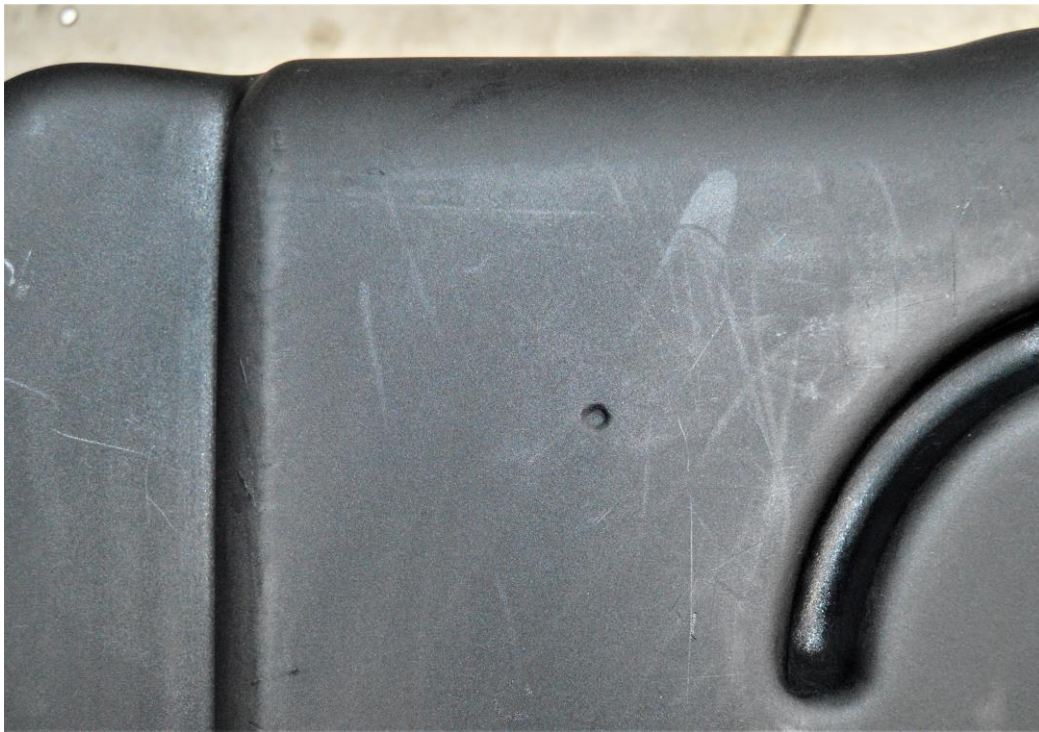
Small indent mark on the bottom of the tank indicates the optimal spot for sump installation of an aftermarket "performance" fuel pump system
