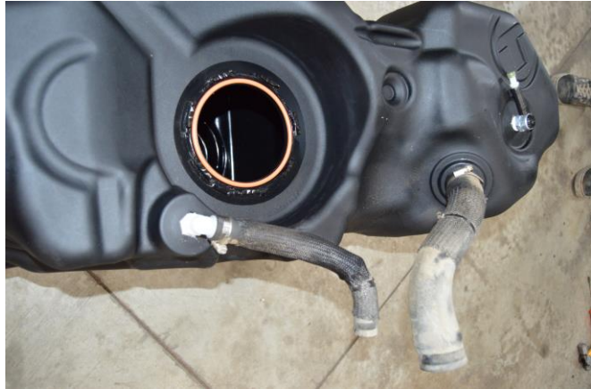
(Fig. 6) Install fill and vent hoses from original equipment tank on TITAN tank as shown. Make sure that they are lined up with orientation marks on the tank.
