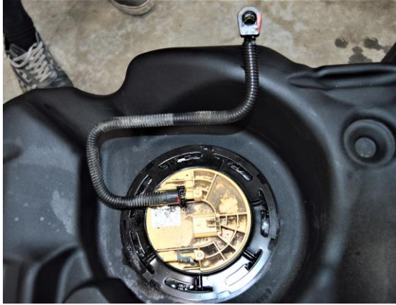
(Fig. 5) Using a hammer and punch, or screwdriver tighten the locking top ring clockwise. The short feed line is shown installed in photo.
