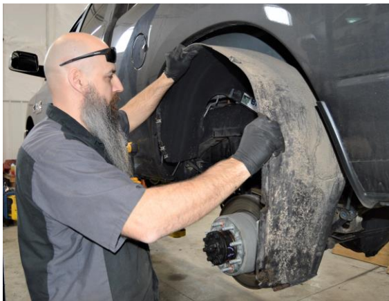
(Fig. 1) Remove driver's side rear wheel and fender liner.
