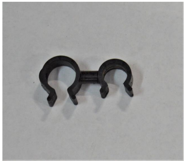
(Fig. 8) Remove the hose clip from the lines leading to the sending unit. Clip shown above.
