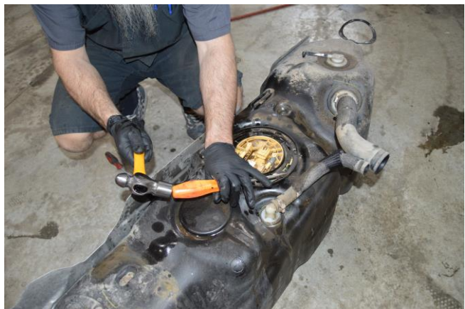
(Fig. 2) Loosen locking top ring on original equipment tank by tapping counter-clockwise, remove and lift out sending unit.
