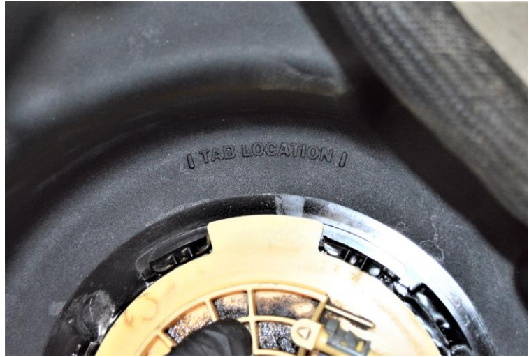
(Fig. 4) Line the sending unit tab up with the "TAB LOCATION" marking on the tank.
