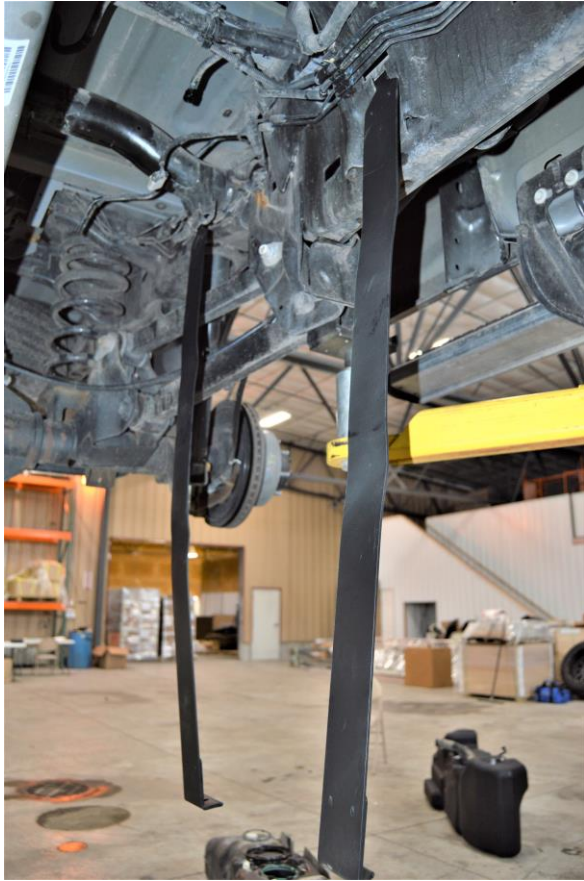
(Fig. 7) Hang the straps in the “T” brackets on the outboard side. Straighten the straps as shown.
