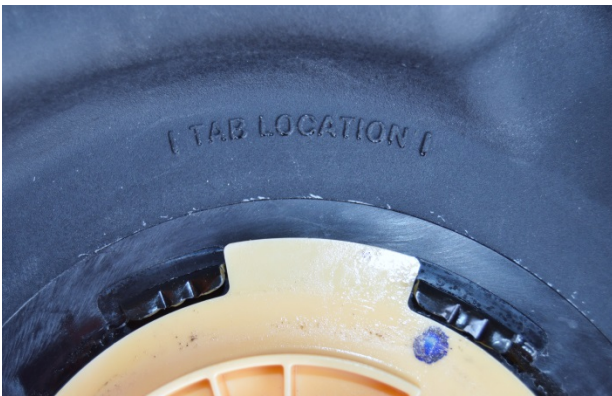
(Fig. 4) Be sure the tab on the sending unit lines up with the “TAB LOCATION” marks on the tank body as shown above.
