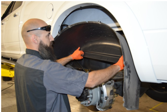
(Fig. 1) Some vehicles may require the removal of the fender liner and perhaps the left rear wheel so as to facilitate access to the tank fill and vent hoses.
