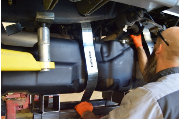
(Fig. 12) You might want to straighten the tank straps a little to aid in installation.
