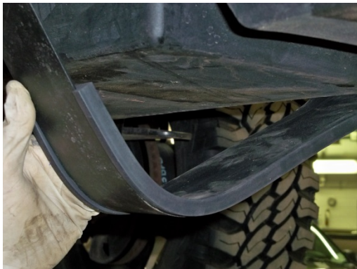
(Fig. 5) If optional TITAN Shield is not to be installed, place rubber bushings (pn 99 0000 0103) on both straps and the Front Support with the channel side toward the strap.
