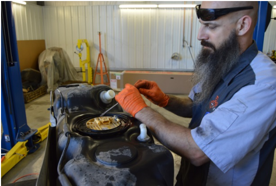
(Fig. 2) Loosen the hold-down ring on the OEM tank by turning counter-clockwise. Note where the connections on your vehicle’s sending unit are “clocked” and install so they are located in the same position in the new tank.
