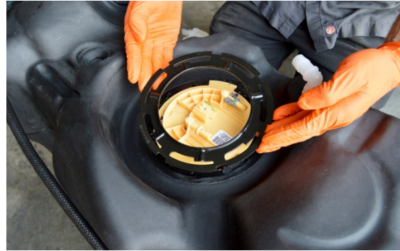
(Fig. 3) Place the sending unit into the TITAN tank and place the Torque Ring hold-down ring on top, threading it onto the lugs. Tighten the ring by turning it clockwise as far as it will go.
