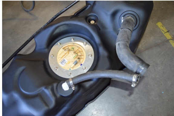
(Fig. 6) Photo shows the fill and main vent hoses transferred and installed on new TITAN tank. Note the 5/16” hose between the two rollover valves. The small line from the vehicle’s fill spout will attach to the tee in this line.
