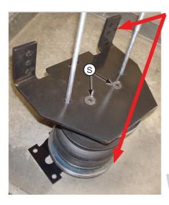
The flanges on the lower bracket must be installed so they are on the opposite side of the fitting that is on the top of the air spring.
