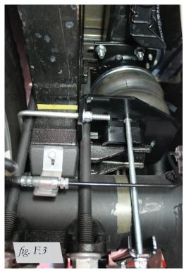
Driver's (left) rear view of kit installed.
