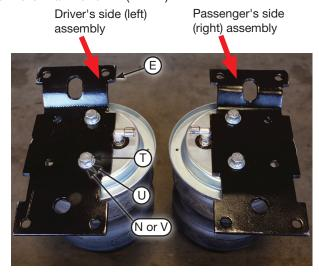
3. Flip the assemblies over and set a roll plate (F) onto the bottom of the air springs (Fig. D.9).
