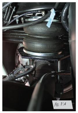
Driver's (left) side inside frame view of kit installed.
