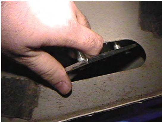
BOLT PLATE INSTALLATION FIGURE 5 INSTALACIÓN DE LA PLACA DE PERNOS, FIGURA 5 INSTALLATION DE LA PLAQUETTE DE BOULON FIGURE 5
