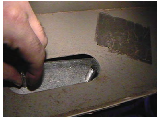
BOLT PLATE INSTALLATION FIGURE 5 INSTALACIÓN DE LA PLACA DE PERNOS, FIGURA 5 INSTALLATION DE LA PLAQUETTE DE BOULON FIGURE 5
