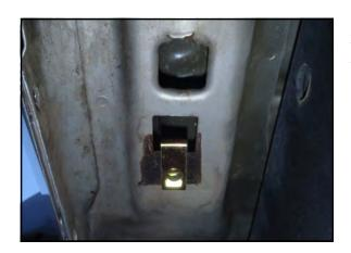
2. Starting at the front driver side mounting location. The bottom rocker mounting hole may be covered by black tape. After removal, insert an M8 clip nut through the square hole. Some vehicles may already be equipped with a threaded hole.
