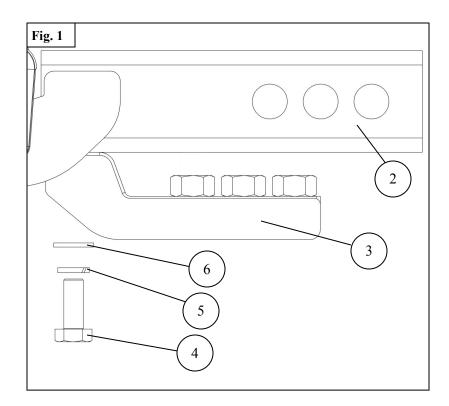
3. Slide the bracket assembly into the receiver hitch of your vehicle. Secure bracket using the receiver pin (not included). *Note:* Secure the bracket assembly as far in the hitch as possible. Three sets of holes have been provided for adjustment.
