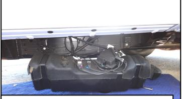
Carefully bring the tank down trying not to tilt or twist the tank to avoid damage to connectors. Note: Trimming might be required on the plastic cover, at the bracket location.
