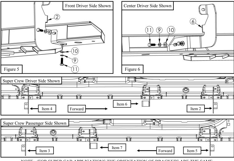
NOTE : (FOR SUPER CAB APPLICATIONS THE ORIENTATION OF BRACKETS ARE THE SAME. THE ONLY DIFFERENCE IS IT WILL **NOT** HAVE CENTER BRACKETS.)
