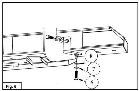
5. Align and adjust the step bars and brackets as needed, then fully tighten all hardware: M8 to 18 ft-lbs, M10 to 38 ft-lbs.
