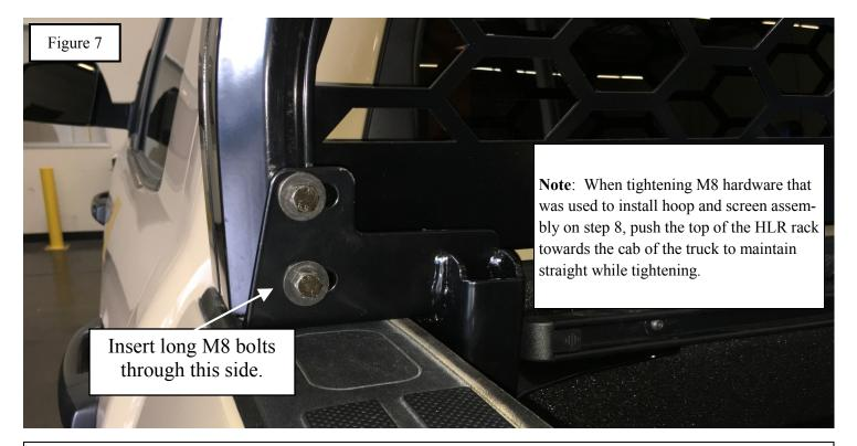
8. Next, position headache rack on brackets and fasten using M8 hardware items 6-8. See Figure 7.
