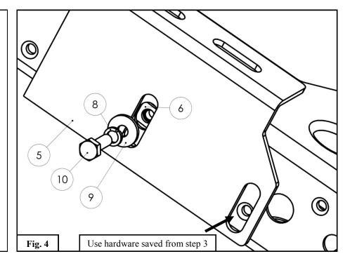
5. Loosely install the support tubes (3 & 4) using the supplied M10 hardware (8-10) according to **Figures 5-7**. *Note*: Driver's side shown in figures 5-7.
