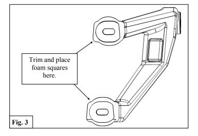
6. Place foam squares on the underside of each cowl mount foot and trim as necessary. See **Figure 3**.
