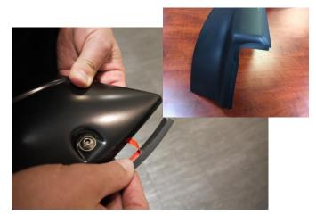
**STEP 1:** Using the supplied alcohol wipes, be sure to clean the inside of the Fender Flare where the rubber seal attaches and wipe away any residue with a dry clean cloth. Peel back 2" of the adhesive backing and position on the Fender Flare. Attach the rubber seal to the Fender Flare, peeling back the red liner a few inches at a time. Ensure pressure is used to secure rubber seal to Fender Flare edge. Attach rubber seal along all areas the Fender Flare will contact the vehicle body.
