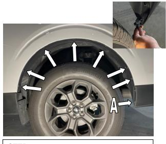
**STEP 4:** Begin by removing factory push-in plugs where noted in image above. Retain for re-install. Using #7 Hex Socket Head, remove lower screw at position "A". Retain for re-install.
