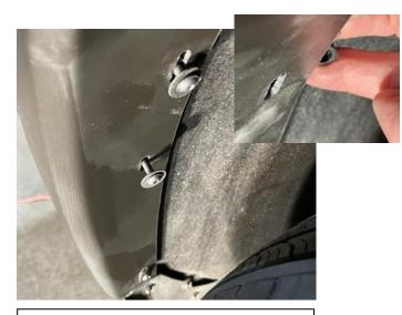
**STEP 7:** Place the smaller of the two-piece front Fender Flare on the vehicle into the position of best fit. Peel back 2" inches of the red tape liner on the fender flare rubber seal at both ends, ensure red liner can be pulled from the outside of the part. Place spacer between wheel liner and Fender Flare. Align the slotted hole in the fender flare with the hole of the spacer and begin to fasten with supplied Allen Head screw.
