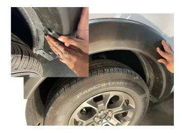
**STEP 6:** Place the larger of the two-piece front Fender Flare on the vehicle into the position of best fit. Peel back 2" inches of the red tape liner on the fender flare rubber seal at both ends, ensure red liner can be pulled from the outside of the part. Begin re-installing the factory push-in plugs at the (5) pre-existing slots in the fender flare.
