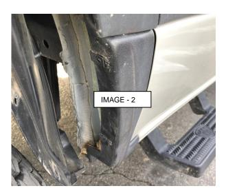
**STEP 5:** Pull the front wheel liner back enough to replace the factory push-on barrel nuts (IMAGE-1) with the supplied push-on barrel nuts (IMAGE-2) where noted in images above. Once installed, place wheel liner back into position.
