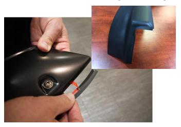
**STEP 9:** Using the supplied alcohol wipes, be sure to clean the inside of the Fender Flare where the rubber seal attaches and wipe away any residue with a dry clean cloth. Peel back 2" of the adhesive backing and position on the Fender Flare. Attach the rubber seal to the Fender Flare, peeling back the red liner a few inches at a time. Ensure pressure is used to secure rubber seal to Fender Flare edge. Attach rubber seal along all areas the Fender Flare will contact the vehicle body.
