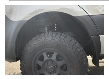
**STEP 3:** Clean the body areas where the Fender Flares will make contact. Ensure fenders are dry prior to install. Turn tires outward for Fender Flare installation.
