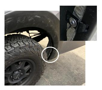
**STEP 13:** Using the supplied clip marked with an "X" and Torx head screw, install at the location circled in the above image.
