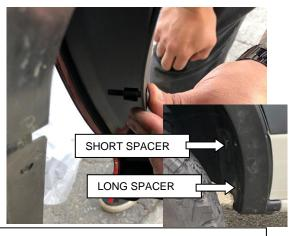
**STEP 7:** Per image above, place spacers in between the fender flare and vehicle, align the slotted hole in the fender flare with the hole of the spacer and begin to fasten with supplied Allen Head screw.
