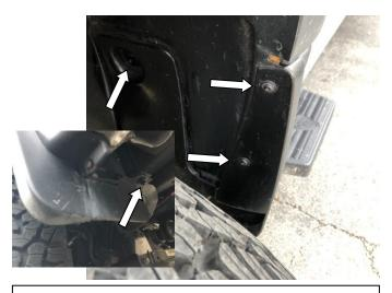
**STEP 4:** Begin by removing factory mud flap using a T-25 TORX and a 10mm socket.
