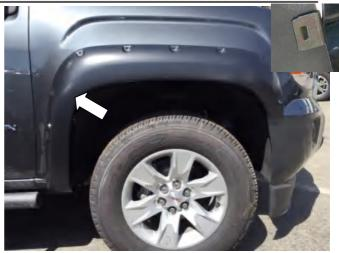
**STEP 7:** Place the Fender Flare onto the vehicle and fit into the correct position following the contours of the body. Use 3 of the retaining clips and previously removed factory screws to secure the Fender Flare to the body using #15 Torx head screwdriver. Make sure the clip securely engages the slots in Fender Flare.
