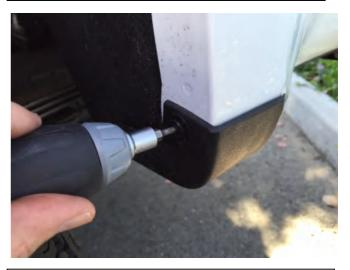
**STEP 6:** Using a #15 Torx head screwdriver remove bottom rear wheel arch molding screw. Maintain screws for re-install.
