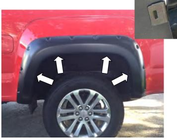
**STEP 13:** Install the provided U shape metal clips at the (4) remaining slot locations in the Fender Flare. Ensure that positive pressure is applied on the Fender Flare to the vehicle fender when installing clips. Slide the clips over the Fender Flare and the inner lip of the wheel arch molding ensuring that the barb in the clip locates in the slot of the Fender Flare.
