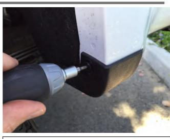
**STEP 11:** Using #15 Torx head screwdriver, remove lower screw from the rear factory deflector. Remove the top factory screw from the front rear deflector. Maintain screws for re-install.
