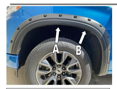
**STEP 7:** Place Fender Flare on the vehicle into the position of best fit. Note where the slots in Fender Flare at positions **A**, **B** and vehicle wheel arch. Remove Fender Flare. Place the small abrasive resistant tapes over the fender lip at the noted positions **A**, **B**. Slide the large clips over the inner fender pannel at the noted **A**, **B** positions, ensure the hook on the back of the clip engages over the fender lip.
