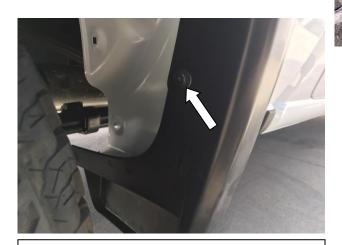
**STEP 17:** Using #15 Torx head screwdriver reinstall the upper screw from the front factory spat in the rear wheel arch through the slot in the Fender flare.
