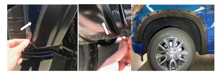
**STEP 10:** Starting at the front of the Fender Flare, carefully remove tape liner from extrusion a few inches at a time. Ensure extrusion is not tucking into flare and sits flush neatly against the fender body. Apply forward pressure to adhere the extrusion along the edge of entire length of Fender Flare once extrusion liner is removed. Ensure all fixing points are tight and secure and that the extrusion is flush neatly against the vehicle body. Repeat install steps for the opposite side.
