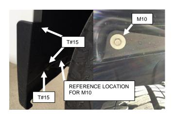
**STEP 5:** For models <u>with front</u> factory mud guards, remove the (3) #15 Torx head screws at the upper and lower screw locations and (1) M10 socket at the underside location indicated above, maintain #15 Torx head screws for re-install. Retain factory mudguards for later use if required, fender flares require the mud guards to be removed.
