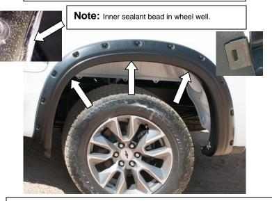
**STEP 18:** To secure the Fender Flare to the body, apply upward tension on Fender Flare to the vehicle fender when installing the black metal clips. Slide the clips over the Fender Flare and the inner wheel arch lip in the three locations shown. Position the clip so that the barb in the clip locates in the slot of the Fender Flare. Ensure all fixing points are tight and secure and that the extrusion is flush neatly against the vehicle body. Repeat install steps for the opposite side.
