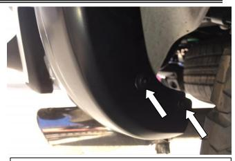
**STEP 16:** Place Fender Flare on the vehicle into the position of best fit. Note where the slots in Fender Flare align with the previously removed factory screws in the front and rear spats. Peel back 2 inches of the red tape liner on the fender flare extrusion at both ends, ensure liner is on the outside of part ref to step 18. Using #15 Torx head screwdriver re-install the upper and lower screws from the rear factory spat through the slots in the Fender Flare.
