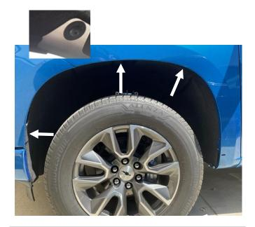
**STEP 6:** Using #15 Torx, proceed to remove the factory screws at the locations noted above. Retain for re-use in steps to follow. Please note: In the image above the mud flap has been removed.
