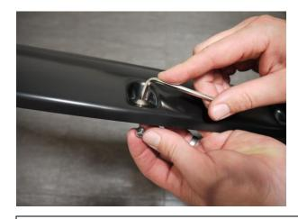
**STEP 1:** Attach the bolts and nuts to each Fender Flare using a 3/16" Allen key/Trox and a 1/2" wrench/socket. wrench/socket. (wrench /socket and Allen key not supplied). Ensure inside of Fender Flares where the rubber seal is attached is clean, using the alcohol wipes provided. Wipe away any residue with a dry clean cloth.
