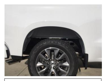
**STEP 13:** Clean the body areas where the Fender Flares will make contact. Ensure fenders are dry prior to install.
