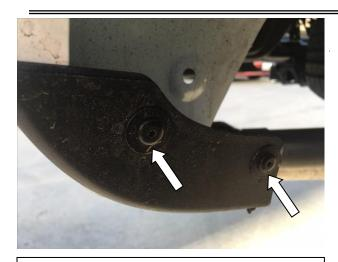
**STEP 15:** Using #15 Torx head screwdriver remove the two botton screws from the rear factory spat. Maintain screws for re-install.
