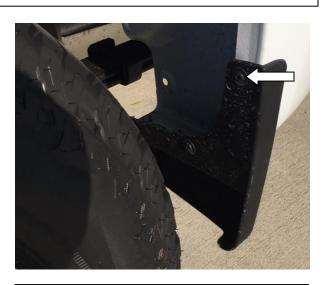
**STEP 14:** Using #15 Torx head screwdriver remove upper screw from the front factory spat in the rear wheel arch. Maintain screws for re-install.
