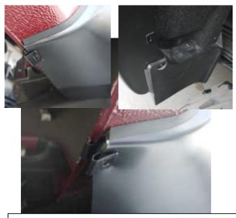
**STEP 11:** Slide the top edge of rear front mudguard cut out behind the factory mudguard. Install the E shape clip so that the clip slides over the inner sheet metal lip and is in line with the slot in the underside of Fender Flare. To secure the clip to Fender Flare apply inward tension on Fender Flare to the vehicle fender when installing the E clip, position the clip so that the barb in the clip locates in the slot of the Fender Flare.
