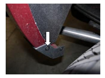
**STEP 9:** Using #15 Torx head screwdriver remove upper screw from the rear factory mudguard. Maintain screws for re-install.
