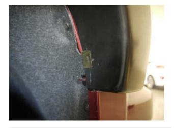
**STEP 7:** To secure the front slot in the Fender Flare to the body, take the black metal clip and slide it over the Fender Flare and the inner wheel arch lip. Position the clip so that the barb in the clip locates in the slot of the Fender Flare. Ensure all fixing points are tight and secure and that the rubber seal is flush neatly against the vehicle body.
