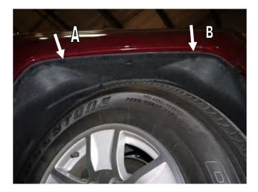
**STEP 2:** Place Fender Flare on the vehicle into the position of best fit. Note where the slots in Fender Flare at positions **A** and **B** align with the existing screws in the vehicle wheel arch. Remove Fender Flare. Remove the existing vehicle screws in location **A** and **B** using #15 Torx head screwdriver. Maintain screws for re-install.
