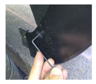
**STEP 12:** Using #15 Torx head screwdriver reinstall the upper screw from the rear factory mudguard through the slot in the Fender Flare. Ensure all fixing points are tight and secure and that the rubber seal is flush neatly against the vehicle body.
