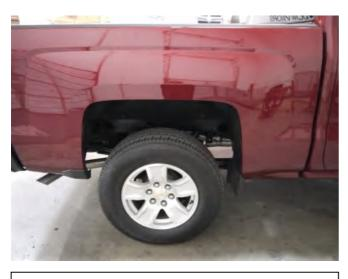
**STEP 8:** Clean the body areas where the Fender Flares will make contact. Ensure fenders are dry prior to install.
