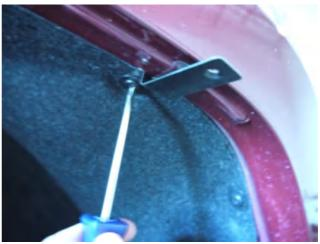
**STEP 4:** Apply clear tape to the inside edge of the fender wheel arch in front of positions **A** and **B** (step 5) over mastic sealant. Install the large brackets in positions **A** and **B** (step 5) aligning the slot in the bracket with the vacant holes from the factory screws in the vehicle wheel arch. Ensure clips are positioned over the clear tape. Reinstall the factory screws in location **A** and **B** using a #15 Torx head screwdriver.
