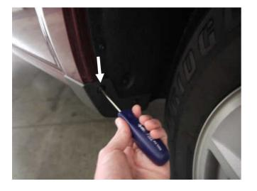
**STEP 3:** Using #15 Torx head screwdriver remove upper screw from the front factory mudguard. Maintain screws for re-install.
