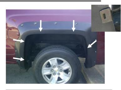
**STEP 10:** To secure the Fender Flare to the body, apply upward tension on Fender Flare to the vehicle fender when installing the black metal clips. Slide the clips over the Fender Flare and the inner wheel arch lip in the five locations shown. Position the clip so that the barb in the clip locates in the slot of the Fender Flare.
