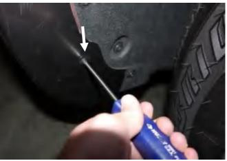
**STEP 6:** Re-install factory screw in the mudguard using #15 Torx head screwdriver through the slot in the Fender Flare.
