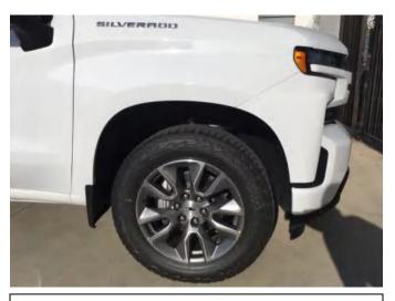
**STEP 4:** Clean the body areas where the Fender Flares will make contact. Ensure fenders are dry prior to install. Turn tires outward for Fender Flare installation.
