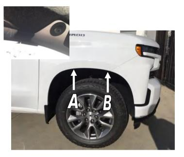
**STEP 6:** Place Fender Flare on the vehicle into the position of best fit. Note where the slots in Fender Flare at positions **A**, **B** and vehicle wheel arch. Remove Fender Flare. Place the small abrasive resistant tapes over the fender lip at the noted posistions **A**, **B**. Slide the large clips over the inner fender pannel at the noted **A**, **B** positions, ensure the hook on the back of the clip engages over the fender lip.
