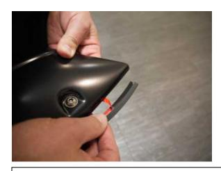
**STEP 2:** Attach the included rubber seal to the Fender Flares. Peel back 2" of the adhesive backing and position on the Fender Flare. Attach the seal to the Fender Flare, peeling back a few inches at a time. Ensure pressure is used to secure rubber seal to Fender Flare edge. Attach rubber seal along all areas the Fender Flare will make contact with the vehicle body.
