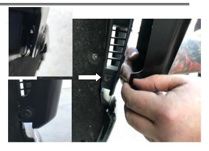
**STEP 7:** Place Fender Flare on the vehicle into the position of best fit. Using #15 Torx head screwdriver reinstall previously removed factory mudguard screws at the upper and lower screw locations through the slots in the Fender Flare at the two noted locations. At the noted **A**, **B** positions secure the Fender Flare to the wheel arch by ensuring the notch in clip locates securely into the slot in the Fender Flare.
