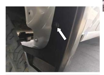
**STEP 16:** Using #15 Torx head screwdriver reinstall the upper screw from the front factory spat in the rear wheel arch through the slot in the Fender flare.
