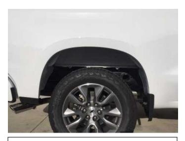
**STEP 12:** Clean the body areas where the Fender Flares will make contact. Ensure fenders are dry prior to install.
