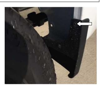
**STEP 13:** Using #15 Torx head screwdriver remove upper screw from the front factory spat in the rear wheel arch. Maintain screws for re-install.
