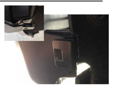
**STEP 8:** Place the small abrasive resistant tape over the inner bumper pannel at the slot location in the front of the fender flare. Install the E shape clip so that the clip slides over the inner bumper pannel lip and is in line with the slot in the Fender Flare. To secure the clip to Fender Flare apply inward tension on Fender Flare to the vehicle fender when installing the E clip, position the clip so that the notch in the clip locates securely in the slot of the Fender Flare.
