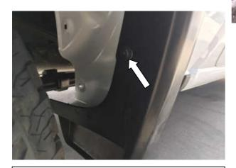
**STEP 16:** Using #15 Torx head screwdriver reinstall the upper screw from the front factory spat in the rear wheel arch through the slot in the Fender flare.
