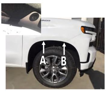
**STEP 6:** Place Fender Flare on the vehicle into the position of best fit. Note where the slots in Fender Flare at positions **A**, **B** and vehicle wheel arch. Remove Fender Flare. Place the small abrasive resistant tapes over the fender lip at the noted positions **A**, **B**. Slide the large clips over the inner fender pannel at the noted **A**, **B** positions, ensure the hook on the back of the clip engages over the fender lip.
