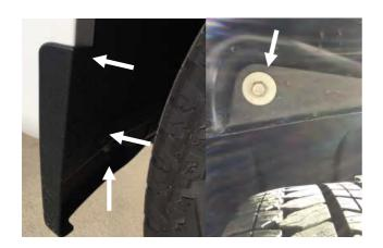
**STEP 5:** For models <u>with front</u> factory mud guards, remove using #15 Torx head screwdriver at the upper and lower screw locations from the front factory mudguards and M10 socket at the underside location indicated above, maintain #15 Torx head screws for re-install. Retain factory mudguards for later use if required, fender flares require the mud guards to be removed.
