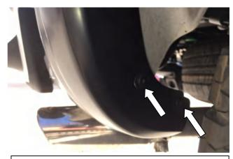
**STEP 15:** Place Fender Flare on the vehicle into the position of best fit. Note where the slots in Fender Flare align with the previously removed factory screws in the front and rear spats. Using #15 Torx head screwdriver re-install the upper and lower screws from the rear factory spat through the slots in the Fender Flare.
