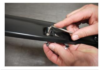
**STEP 10:** Attach the bolts and nuts to each Fender Flare using 3/16" Allen key/Trox and a 1/2" wrench/socket. wrench/socket. (wrench /socket and Allen key not supplied). Ensure inside of Fender Flares where the rubber seal is attached is clean, using the alcohol wipes provided. Wipe away any residue with a dry clean cloth.
