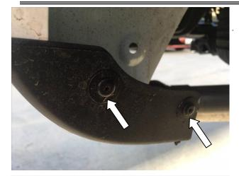
**STEP 14:** Using #15 Torx head screwdriver remove the two botton screws from the rear factory spat. Maintain screws for re-install.
