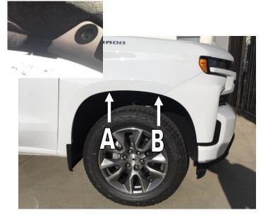
**STEP 6:** Place Fender Flare on the vehicle into the position of best fit. Note where the slots in Fender Flare at positions **A**, **B** and vehicle wheel arch. Remove Fender Flare. Place the small abrasive resistant tapes over the fender lip at the noted posistions **A**, **B**. Slide the large clips over the inner fender pannel at the noted **A**, **B** positions, ensure the hook on the back of the clip engages over the fender lip.
