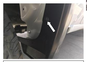
**STEP 16:** Using #15 Torx head screwdriver reinstall the upper screw from the front factory spat in the rear wheel arch through the slot in the Fender flare. **Note:** Inner sealant bead in wheel well.
