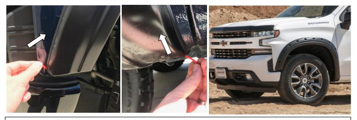
**STEP 9:** Starting at the front of the Fender Flare, carefully remove tape liner from extrusion a few inches at a time. Ensure extrusion is not tucking into flare and sits flush neatly against the fender body. Apply forward pressure to adhere the extrusion along the edge of entire length of Fender Flare once extrusion liner is removed. Ensure all fixing points are tight and secure and that the extrusion is flush neatly against the vehicle body. Repeat install steps for the opposite side.
