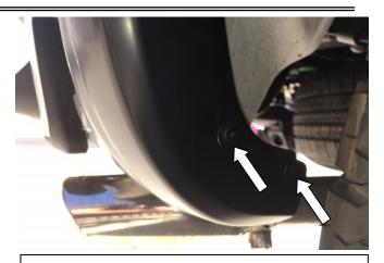
**STEP 15:** Place Fender Flare on the vehicle into the position of best fit. Note where the slots in Fender Flare align with the previously removed factory screws in the front and rear spats. Peel back 2 inches of the red tape liner on the fender flare extrusion at both ends, ensure liner is on the outside of part ref to step 18.Using #15 Torx head screwdriver re-install the upper and lower screws from the rear factory spat through the slots in the Fender Flare.
