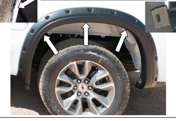
**STEP 17:** To secure the Fender Flare to the body, apply upward tension on Fender Flare to the vehicle fender when installing the black metal clips. Slide the clips over the Fender Flare and the inner wheel arch lip in the three locations shown. Position the clip so that the barb in the clip locates in the slot of the Fender Flare. Ensure all fixing points are tight and secure and that the extrusion is flush neatly against the vehicle body. Repeat install steps for the opposite side.
