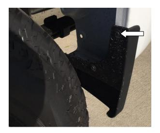
**STEP 13:** Using #15 Torx head screwdriver remove upper screw from the front factory spat in the rear wheel arch. Maintain screws for re-install.
