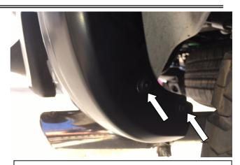
**STEP 15:** Place Fender Flare on the vehicle into the position of best fit. Note where the slots in Fender Flare align with the previously removed factory screws in the front and rear spats. Peel back 2 inches of the red tape liner on the fender flare extrusion at both ends, ensure liner is on the outside of part ref to step 18.Using #15 Torx head screwdriver re-install the upper and lower screws from the rear factory spat through the slots in the Fender Flare.
