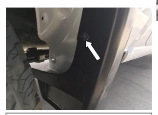
**STEP 16:** Using #15 Torx head screwdriver reinstall the upper screw from the front factory spat in the rear wheel arch through the slot in the Fender flare. Note: Inner sealant bead in wheel well.
