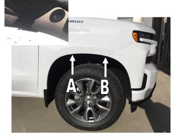
**STEP 6:** Place Fender Flare on the vehicle into the position of best fit. Note where the slots in Fender Flare at positions **A**, **B** and vehicle wheel arch. Remove Fender Flare. Place the small abrasive resistant tapes over the fender lip at the noted posistions **A**, **B**. Slide the large clips over the inner fender pannel at the noted **A**, **B** positions, ensure the hook on the back of the clip engages over the fender lip.
