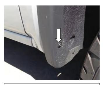
**STEP 3:** Using #15 Torx head screwdriver remove bottom rear wheel arch molding screw. Maintain screws for re-install.
