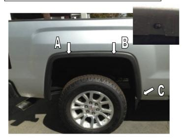
**STEP 9:** Place Fender Flare on the vehicle into the position of best fit. Note where the slots in Fender Flare at positions **A** and **B** align with the existing screws in the vehicle wheel arch molding. Also note where the slot in the Fender Flare aligns with the front mud flap deflector, position **C**. Remove Fender Flare. Remove the existing vehicle screws in location **A** and **B** using #15 Torx head screwdriver. Maintain screws for re-install.
