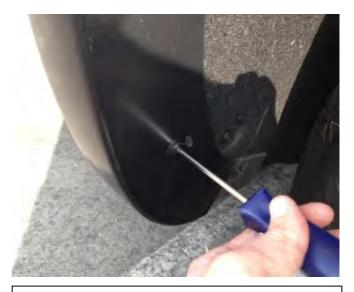
**STEP 6:** Loosely re-install previously removed factory screw through the slot in the Fender Flare at the bottom rear wheel arch molding using #15 Torx head screwdriver.
