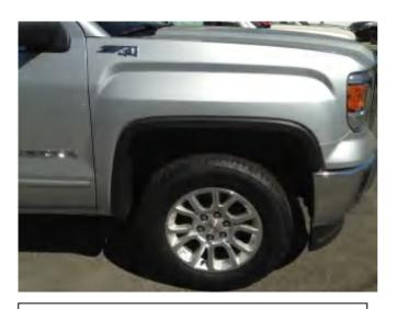
**STEP 1:** Clean the body areas where the Fender Flares will make contact. Ensure fenders are dry prior to install. Turning tires outward during install of each Fender Flare will ensure ease of install at bottom fixing points.
