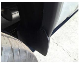
**STEP 10:** Using #15 Torx head screwdriver, remove upper screw as previously noted in position **C** from the factory mud flap deflector. Maintain screws for re-install.
