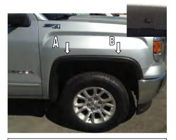
**STEP 2:** Place Fender Flare on the vehicle into the position of best fit. Note where (4) slots in Fender Flare correspond with (4) existing screws in the vehicle wheel arch molding. Remove Fender Flare. Remove the existing vehicle screws in location **A** and **B** using #15 Torx head screwdriver. Maintain screws for re-install.
