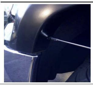
**STEP 7:** Loosely re-install factory screw through the remaining slot in the front upper wheel arch molding. Ensure Fender Flare is centered and in position of best fit on fender. Tighten all front fender fixing points to ensure a tight and secure fit and that the rubber seal is flush neatly against the vehicle body.
