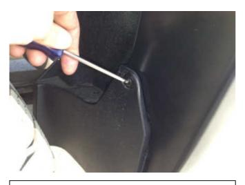
**STEP 11:** Place Fender Flare on the vehicle into the position of best fit, slide the bottom front end of Fender Flare between the existing mud flap deflector and wheel arch molding so that the slot in the Fender Flare is under the vacant hole in the mud flap. Using #15 Torx head screwdriver, loosely re-install the previously removed screw. Ensure the installed rubber seal from is resting firmly on the mud flap deflector.
