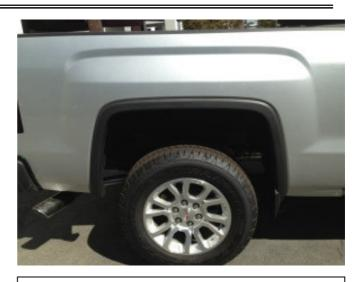
**STEP 8:** Clean the body area where the Fender Flares will make contact. Ensure fenders are dry prior to install.
