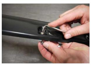
**STEP 10:** Attach the bolts and nuts to each Fender Flare using 3/16" Allen key/Trox and a 1/2" wrench/socket. wrench/socket. (wrench /socket and Allen key not supplied). Ensure inside of Fender Flares where the rubber seal is attached is clean, using the alcohol wipes provided. Wipe away any residue with a dry clean cloth.
