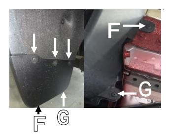
**STEP 14:** Using #15 Torx head screwdriver remove the two botton screws from the rear factory spat. Maintain screws for re-install.
