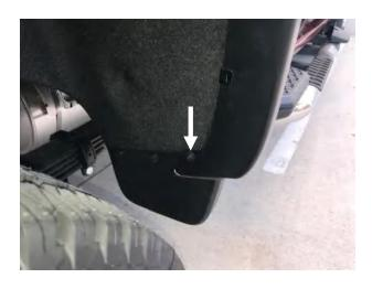
**STEP 16:** Using #15 Torx head screwdriver reinstall the upper screw from the front factory spat in the rear wheel arch through the slot in the Fender flare.
