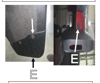
**STEP 13:** Using #15 Torx head screwdriver remove the upper and lower (**E**) screw from the front factory spat in the rear wheel arch. Maintain screws for re-install.
