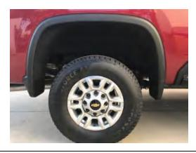
**STEP 15:** Place Fender Flare on the vehicle into the position of best fit. Note where the slots in Fender Flare align with the previously removed factory screws in the front and rear spats. Using #15 Torx head screwdriver re-install the upper and lower screws from the rear factory spat through the slots in the Fender Flare.
