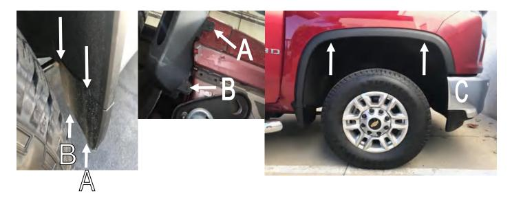
**STEP 5:** For models <u>with front</u> factory mud guards, remove using #15 Torx head screwdriver at the upper x2 and lower (A and B) screw locations from the front factory mudguards and M10 socket at the underside location indicated above, maintain #15 Torx head screws for reinstall. Retain factory mudguards for later use if required, fender flares require the mud guards to be removed.
