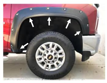
**STEP 7:** Place Fender Flare on the vehicle into the position of best fit. Using #15 Torx head screwdriver reinstall previously removed factory mudguard screws at the upper and lower screw locations through the slots in the Fender Flare at the two noted locations. At the noted **C**, **D** positions secure the Fender Flare to the wheel arch by ensuring the notch in clip locates securely into the slot in the Fender Flare.
