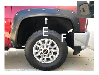
**STEP 8:** At the noted **E**, **F** positions secure the Fender Flare to the wheel arch by ensuring the notch in clip locates securely into the slot in the Fender Flare.
