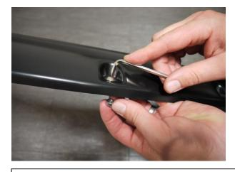
**STEP 1:** Attach the bolts and nuts to each Fender Flare using a 3/16" Allen key/Trox and a 1/2" wrench/socket. (wrench /socket and Allen key not supplied). Ensure inside of Fender Flares where the rubber seal is attached is clean, using the alcohol wipes provided. Wipe away any residue with a dry clean cloth.
