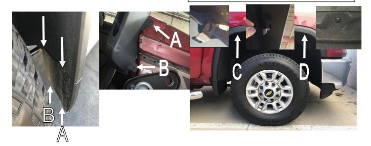
**STEP 5:** For models with front factory mud guards, remove factory Torx screw using #15 Torx head screwdriver at the upper x2 and lower (A and B) screw locations. Maintain #15 Torx head screws for re-install. Retain factory mudguards for later use if required, fender flares require the mud guards to be removed.
