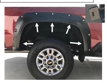
**STEP 17:** To secure the Fender Flare to the body, apply upward tension on Fender Flare to the vehicle fender when installing the black metal clips. Slide the clips over the Fender Flare and the inner wheel arch lip in the five locations shown. Position the clip so that the barb in the clip locates in the slot of the Fender Flare. Ensure all fixing points are tight and secure and that the rubber seal is flush neatly against the vehicle body. Repeat install steps for the opposite side.
