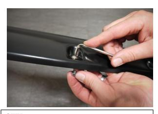
**STEP 9:** Attach the bolts and nuts to each Fender Flare using 3/16" Allen key/Trox and a 1/2" wrench/socket. (wrench /socket and Allen key not supplied). Ensure inside of Fender Flares where the rubber seal is attached is clean, using the alcohol wipes provided. Wipe away any residue with a dry clean cloth.
