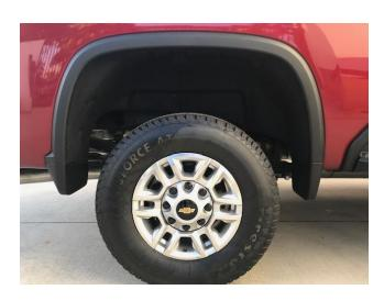
**STEP 11:** Clean the body areas where the Fender Flares will make contact. Ensure fenders are dry prior to install. DO NOT REMOVE THE FACTORY FLARES, the EGR FENDER FLARE was designed to fit directly over the factory
