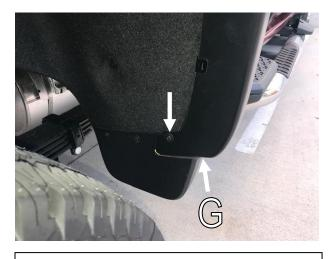
**STEP 16:** Using #15 Torx head screwdriver reinstall the previously removed factory mudguard screws at the upper and lower (G) screw locations through the slots in the front of the Fender Flare at the two noted locations.
