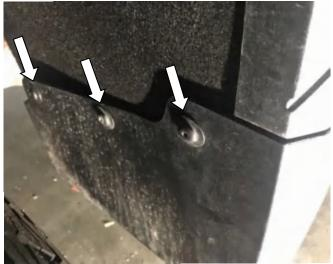
**STEP 12:** Using #15 Torx head screwdriver remove the three screws from the rear factory mud guard in the rear wheel arch. Fender flares require the rear mud guards to be removed, maintain screws for re-install if required.
