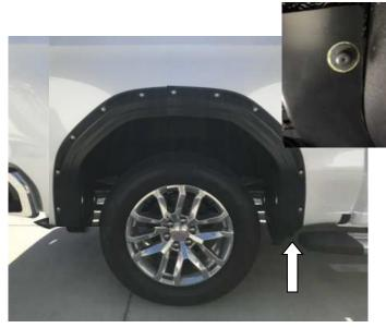
**STEP 14:** Place Fender Flare on the vehicle into the position of best fit. Note where the slot in Fender Flare aligns with the previously removed factory screws in the front and rear spats. Using #15 Torx head screwdriver re-install the screw from the front of the rear factory spat through the slots in the Fender Flare.
