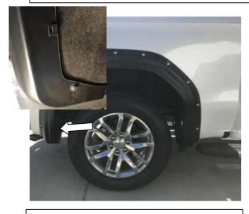
**STEP 15:** Using #15 Torx head screwdriver reinstall the previously removed factory mudguard screws at the upper screw locations through the slots in the front of the Fender Flare at the noted location.
