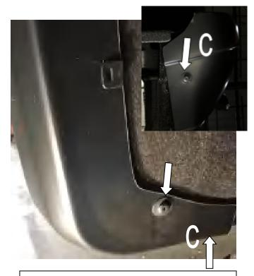
**STEP 7:** Using #15 Torx head screwdriver reinstall the previously removed factory mudguard screws at the upper and lower **(C)** screw locations through the slots in the front of the Fender Flare at the two noted locations.
