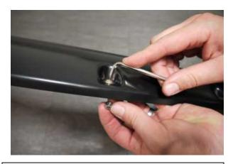
**STEP 9:** Attach the bolts and nuts to each Fender Flare using 3/16" Allen key/Trox and a 1/2" wrench/socket. wrench/socket. (wrench /socket and Allen key not supplied). Ensure inside of Fender Flares where the rubber seal is attached is clean, using the alcohol wipes provided. Wipe away any residue with a dry clean cloth.
