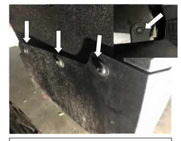
**STEP 5:** Using #15 Torx head screwdriver remove the three factory screws from the front mudguards and one underside screw location, maintain screws for re-install . Fender flares require the mud guards to be removed. Retain factory mudguards for later use if required.
