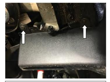
**STEP 13:** Using #15 Torx head screwdriver remove the upper and lower screws from the underside of the rear factory spat in the rear wheel arch. Maintain screws for reinstall. On the front spat using #15 Torx head screwdriver remove the lower screw from the underside that aligns with the slot in the Fender Flare.
