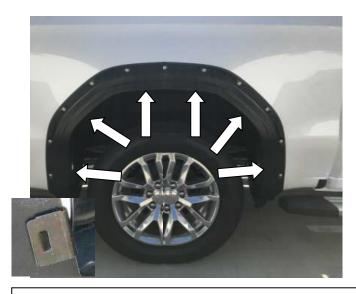
**STEP 16:** To secure the Fender Flare to the body, apply upward tension on Fender Flare to the vehicle fender when installing the large U clips. Slide the clips over the Fender Flare and the inner wheel arch lip in the six locations shown. Position the clip so that the barb in the clip locates in the slot of the Fender Flare. Ensure all fixing points are tight and secure and that the rubber seal is flush neatly against the vehicle body. Repeat install steps for the opposite side.
