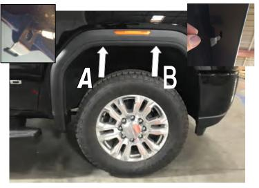
**STEP 6:** Using #15 Torx screwdriver remove factory screws at location **A** and **B**. Place Fender Flare on the vehicle into the position of best fit. Note where the slots in Fender Flare at positions **A**, **B** and vehicle wheel arch are located. Install the large clips to the inner wheel arch by sliding clips into the Fender Flare slots, ensure notch in the clip locates securely into the Fender Flare slot. Re-install the factory screws through the hole in the clips to the wheel arch.
