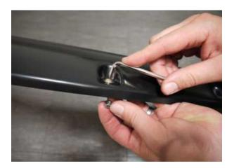
**STEP 1:** Attach the bolts and nuts to each Fender Flare using a 3/16" Allen key/Trox and a 1/2" wrench/socket. wrench/socket. (wrench /socket and Allen key not supplied). Ensure inside of Fender Flares where the rubber seal is attached is clean, using the alcohol wipes provided. Wipe away any residue with a dry clean cloth.
