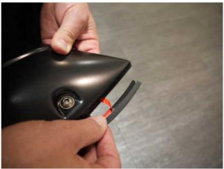
**STEP 13:** Attach the included rubber seal to the Fender Flares. Peel back 2" of the adhesive backing and position on the Fender Flare. Attach the seal to the fender flare, peeling back a few inches at a time. Attach rubber seal along all areas the Fender Flare will make contact with the vehicle body. Trim any excess rubber seal.
