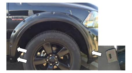
**STEP 11:** Re-install the x2 previously removed screws from STEP 7 using 8.0mm socket. To secure the front slot in the Fender Flare to the body, take the black metal clip and slide it over the Fender Flare and the front bumper lip. Position the clip so that the barb in the clip locates in the slot of the Fender Flare. Ensure all fixing points are tight and secure and that the rubber seal is flush neatly against the vehicle body.
