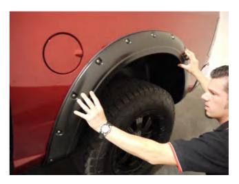
**STEP 15:** Remove all factory bolts using 8.0mm socket and retain for installation of Fender Flares. Place the Fender Flares on to the vehicle and fit into the correct position following the contours of the body.
