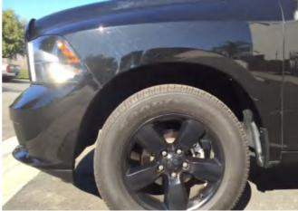
**STEP 6:** Clean the body areas where the Fender Flares will make contact. For models equipped with factory fender flares, removal of factory flares is required, please consult the vehicle service manual for factory fender flare removal.
