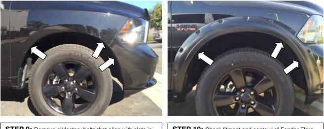
**STEP 9:** Remove all factory bolts that align with slots in part as shown using 8.0mm socket, retain screws for installation of Fender Flares.
