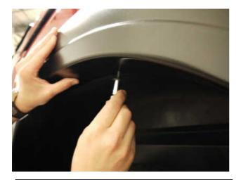
**STEP 16:** Re-install all bolts removed in step 14 using 8.0mm socket.
