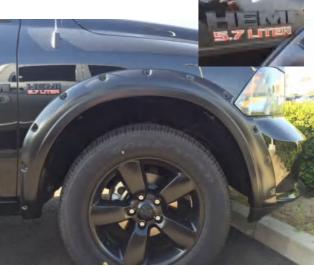
**STEP 8:** Place the Fender Flare onto the vehicle and fit into the correct position following the contours of the body. Vehicle badge may need to be removed and relocated if interference occurs with Fender Flare.
