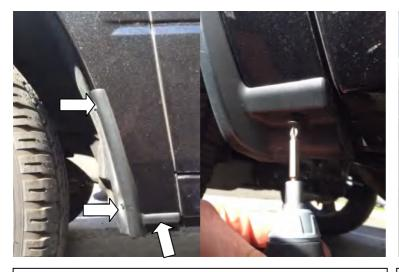
**STEP 7:** If vehicle is equipped with factory splash guard, remove the screw from underside of guard using Phillips head screwdriver. Use 8.0mm socket to remove the x2 screws from inside edge of the splash guard and retain. Splash guard will not work with Fender Flare installation.
