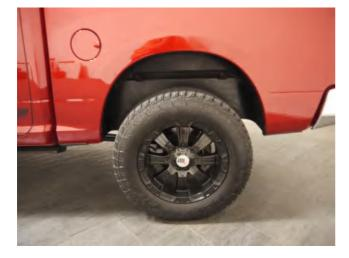
**STEP 14:** Clean the body areas where the Fender Flares will makes contact.. For models equipped with factory fender flares, removal of factory flares is required, please consult the vehicle service manual for factory fender flare removal.
