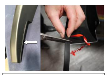
**STEP 3:** Attach rubber seal to the bottom front corner of front and rear Fender Flares per the attached image that will locate around the factory spats. Trim any excess gasket and discard.
