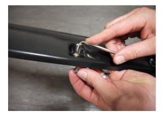
**STEP 1:** Attach the bolts and nuts to each Fender Flare using a 3/16" Allen key and a 10mm wrench/socket (wrench/socket and Allen key not supplied). Ensure inside of Fender Flares where the gasket is attached is clean, using the alcohol wipes provided. Wipe away any residue with a dry clean cloth.
