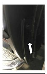
**STEP 7:** Starting at the front of the Fender Flare, carefully remove tape liner from rubber gasket a few inches at a time. Ensure rubber gasket is not tucking into flare and sits flush neatly against the fender body. Ensure all fixing points are tight and secure. Apply forward pressure to adhere the gasket along the edge of entire length of Fender Flare once gasket liner is removed. Repeat install steps for the opposite side of the Fender Flares.
