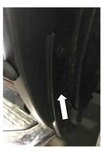
**STEP 12:** Starting at the front of the Fender Flare, carefully remove tape liner from rubber gasket a few inches at a time. Ensure rubber gasket is not tucking into flare and sits flush neatly against the fender body. Ensure all fixing points are tight and secure. Apply forward pressure to adhere the gasket along the edge of entire length of Fender Flare once gasket liner is removed. Repeat install steps for the opposite side of the Fender Flares.
