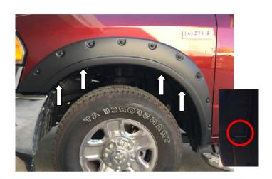
**STEP 6:** Using the previously removed hex head screws, <u>loosely install</u> flares beginning at the front of the flare working to rear. Ensure the cut-out shape fits around factory mud spat against vehicle surface. Ensure the previously removed one inch of tape liner from front and rear Fender Flares is on the outside of the rubber gasket. When satisfied with position, <u>completely</u> <u>secure</u> the (4) hex screws.
