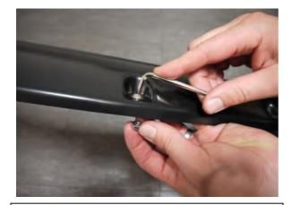
**STEP 1:** Attach the bolts and nuts to each Fender Flare using a 3/16" Allen key and a 10mm wrench/socket (wrench /socket and Allen key not supplied). Ensure inside of Fender Flares where the rubber seal is attached is clean, using the alcohol wipes provided. Wipe away any residue with a dry clean cloth.
