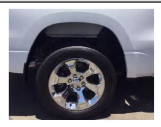
**STEP 7:** Clean the body areas where the Fender Flares will make contact. Ensure fenders are dry prior to install.
