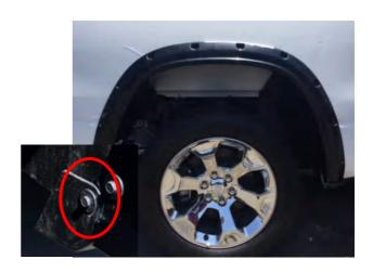
**STEP 10:** Position Fender Flare so that the top (3) slots engage with the raised heads of the grey screw plugs. Using philips head screws, <u>loosely install</u> flare into postion. Using previously removed hex screws, <u>loosely install</u> remaining (5) screws at location (A). Ensure cut out in flare fits around factory mud spat. When satisfied, <u>completely secure</u> the (8) locations.
