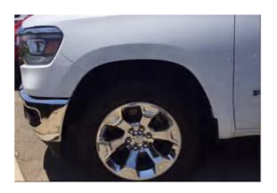
**STEP 4:** Clean the body areas where the Fender Flares will make contact. Ensure fenders are dry prior to install.
