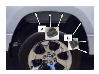
**STEP 9:** Insert grey screw plug into vacant holes at position (A) ensuring that the raised head of the screw plug runs parallel with vehicle body.
