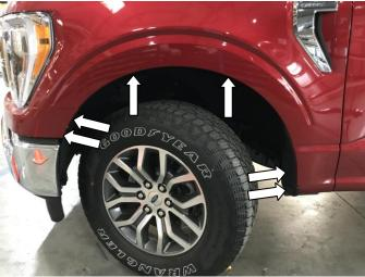
**STEP 6:** Locate six 7mm bolts in the vehicle wheel well.
