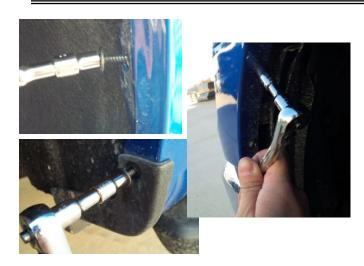
**STEP 7:** Remove six 7mm bolt, retain for installation of Fender Flares.
