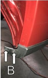
**STEP 12:** Remove the two 7mm factory wheel well spat bolts (A) and the two rear factory retainer clips (B), retain for installation of Fender Flares. Rentainer clips (B) will need to be removed using needle noise pliers.
