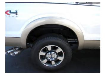
**STEP 5:** Clean the body areas where the Fender Flares will makes contact. Use the supplied alcohol wipe.
