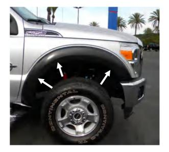
**STEP 4:** Reinstall the 5.5mm socket head screws through slots in the Fender Flare to the vehicle. Make sure the screws are securely engaged to the vehicle fender.
