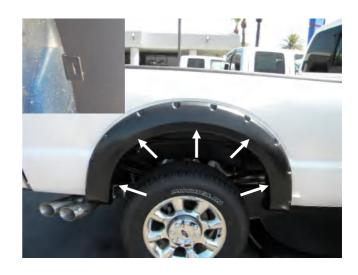
**STEP 6:** Place the Fender Flare onto the vehicle and fit into the correct position following the contours of the body. Use ten (10) of the .6mm clips (five 5 per side) to secure the Fender Flare to the body. Make sure the dimple in the clip securely attaches in the slot on the Fender Flare.
