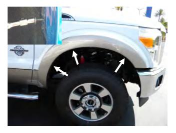
**STEP 2:** Remove all 5.5mm socket head screws and retain for installation of Fender Flares.
