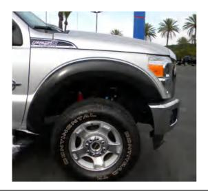
**STEP 3:** Place the Fender Flare onto the vehicle and fit into the correct position following the contours of the body. Ensure the slots in the part align with the holes in the fender from the previously removed 5.5mm socket head screws.
