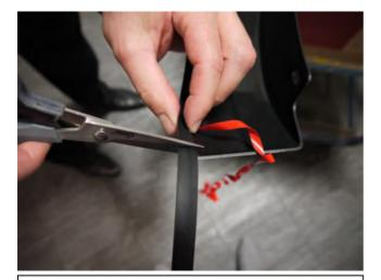
STEP 3: Trim any unnecessary extrusion and discard.
