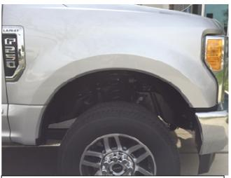
**STEP 4:** Clean the body areas where the Fender Flares will makes contact. A light misting on fender using a soap and water solution can aid in proper rubber placement.
