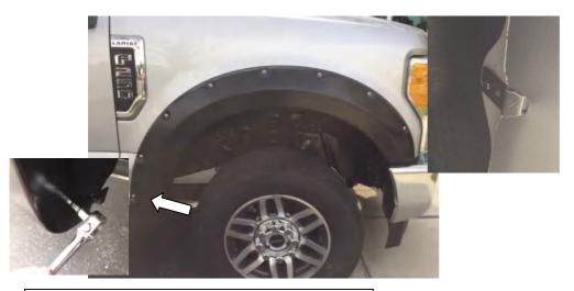
**STEP 7:** Loosely reinstall the lowest rear 7/32" socket head screws through slot in the Fender Flare to the vehicle. Make sure the screws are securely engaged to the vehicle fender. Install provided Long Attachment Clips in remaining four (4) Fender Flare Slots. Loosely reinstall remaining 7/32 in socket head screws. Ensure part is still in the position of best fit and extrusion is in correct position before hand tightening all screws.
