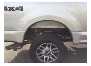
**STEP 10:** Clean the body areas where the Fender Flares will makes contact. A light misting on fender using a soap and water solution can aid in proper rubber placement.
