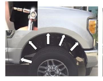
**STEP 5:** Remove all five (5) 7/32" socket head screws and retain for installation of Fender Flares.
