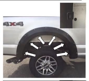
**STEP 11:** Place the Fender Flare onto the vehicle and fit into the correct position following the contours of the body. Use six (6) provided "U" Shaped Retention Clips to secure the Fender Flare to the body. Ensure the barb in the clip securely attaches in the slot on the Fender Flare. REPEAT ALL ABOVE STEPS FOR OPPOSITE SIDE OF VEHICLE.
