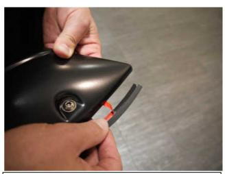
**STEP 2:** Attach the included rubber seal to the Fender Flares. Peel back 2" of the adhesive backing and position on the Fender Flare. Attach the double sided tape to the inside of the Fender Flare, peeling back a few inches at a time. Ensure pressure is used to secure rubber seal to Fender Flare edge. Attach rubber seal along all areas the Fender Flare will make contact with the vehicle body.
