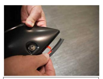
**STEP 9:** Attach the included rubber seal to the Fender Flares. Peel back 2" of the adhesive backing and position on the Fender Flare. Attach the double sided tape to the inside of the Fender Flare, peeling back a few inches at a time. Ensure pressure is used to secure rubber seal to Fender Flare edge. Attach rubber seal along all areas the Fender Flare will make contact with the vehicle body.
