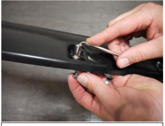
**STEP 1:** Attach the bolts and nuts to each Fender Flare using a 3/16" Allen key and a 10mm wrench/socket (wrench /socket and Allen key not supplied). Ensure inside of Fender Flares where the rubber seal is attached is clean, using the alcohol wipes provided. Wipe away any residue with a dry clean cloth.
