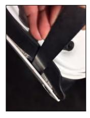
**STEP 20:** At the (4) marked locations on the factory flare in use the Nylon Pry Tool to separate approximately 3/4" either side of the grease pencil mark of the double sided tape that attaches the inner rubber seal to the factory flare.
