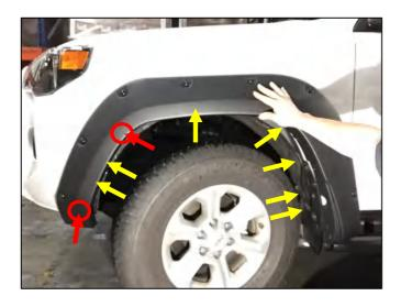
STEP 5: Hold Fender Flare towards the vehicle in position of best fit. Note where slots in Fender Flare wheel arch correspond to existing 10mm hex screws or plastic rivets in wheel arch / mud guard. Remove (9) hex screws from the vehicle. Pay special attention to the (2) circled locations and retain these longer screws for re-installation, discard remaining (7) screws
