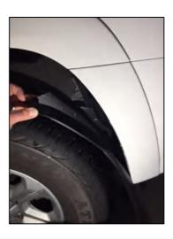
**STEP 15**: Use (L) quarter panel piece to begin install. While pulling mud guard away from vehicle in forward / outward direction, carefully slide the flare between the fender and mud guard so their shapes interlock. Re-install the (1) hex screw previously removed.
