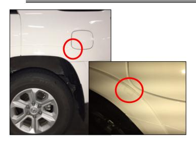
**STEP 14:** Using (1) piece of Mylar Protective Tape apply approximately 1/3 of the length of the tape to the top leading edge of the factory fender flare directly under the corner of the gas cap door. The remaining 2/3 will adhere to the face edge of the factory flare. This will ensure no rubbing contact between factory flare and pocketed flare.
