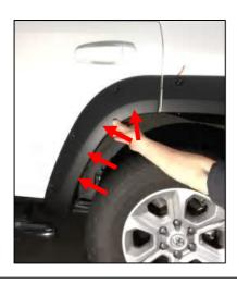
**STEP 18:** Completely remove protective film from outside surface of Fender Flare. Hold Fender Flare towards the vehicle in position of best fit. Note (4) slots in Fender Flare wheel arch.
