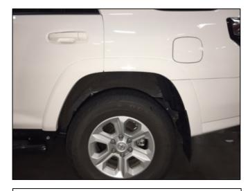
**STEP 10:** Clean the vehicle body areas with a 50/50 Alcohol Mix to remove any dirt and debris where the Fender Flare will make contact with fender.
