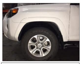
**STEP 4:** Clean the vehicle body areas with a 50/50 soap and water solution to remove any dirt and debris where the Fender Flare will make contact with fender. Re-apply a light misting of 50/50 soap and water solution to aid in gasket installation.
