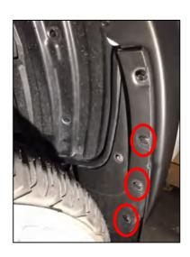
**STEP 17:** At remaining (3) locations in mud guard, reinstall previously removed plastic rivets. Ensure that mud guard is firmly against fender flare and that it is not rolled under in the fender flare cut away shape.
