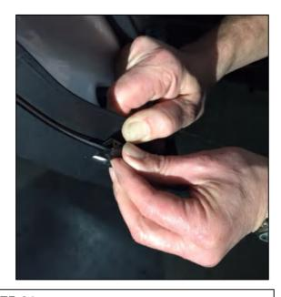
**STEP 24:** When at the 4th installation slot in the Fender Flare door piece, it is important to hold the inner factory rubber seal to support the factory flare. Failure to do this could lead to the factory flare disengaging from the door panel.
