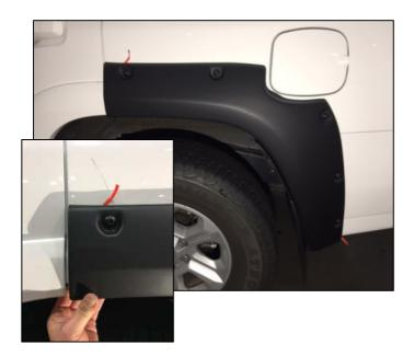
**STEP 16:** Align the Fender Flare even and parallel with the front most edge of the quarter panel and factory flare. Using the (3) provided 10mm Hex Head Screws, install from front to rear in the previously removed screw locations. Ensure that when installing the 3rd screw that it goes through the mud guard to hold mud guard in place.
