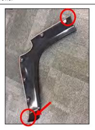
**STEP 13:** Inspect gasket conformity to Fender Flare prior to installation. Rub gasket if needed, to ensure it is not rolled away from edge. Peel back approximately 2" of the double sided tape liner and fold the liner at 45 degrees to the top leading edge of the Fender Flare. Obtain (3) Hex head screws, (5) strips of Mylar Protective Tape and (4) "U" shaped mounting clips from hardware kit.
