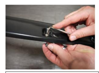
**STEP 1:** Attach the bolts and nuts to each Fender Flare using a 3/16" Allen key and a 1/2" wrench/socket. wrench/socket (wrench /socket and Allen key not supplied). Ensure inside of Fender Flares where the rubber seal is attached is clean, using the alcohol wipes provided. Wipe away any residue with a dry clean cloth.
