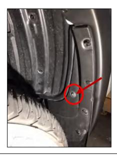
**STEP 12:** In addition to the (3) hex screws removed, remove and retain the inner hex screw of the mud guard shown.
