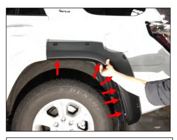
**STEP 11:** Completely remove protective film from outside surface of fender flare. Hold Fender Flare towards the vehicle in position of best fit. Note where slots in Fender Flare wheel arch correspond to existing 10mm hex screws or plastic rivets in wheel arch / mud guard. Remove (3) hex screws and (3) plastic rivets using nylon pry tool. Discard hex screws.
