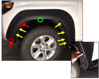
**STEP 7:** Using (1) Mounting Bracket "X", engage bracket into the available slot in the top wheel arch area of the Flare and loosely secure using provided 10mm Hex Screw. Note: Re-inspect gasket to ensure no areas are "rolled under" prior to Installation.
