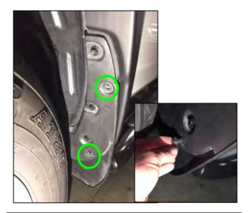
**STEP 9:** Re-install the previously removed (2) plastic retaining rivets into the mud guard. This will complete the installation for front flares. If necessary, apply additional 50/50 soap and water solution for minor adjustments to the flares position and to ensure rubber gasket is flat against the vehicle surface.
