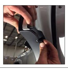
**STEP 23:** Install Fender Flare back into position of best fit on door. Starting at the top slot closest to the previously installed quarter panel piece. Start applying the first (3) "U" Shaped Mounting Clips. It is very important that the factory fender flare is supported when installing these mounting clips. It is also important to ensure that the barb in the "U" Shaped Mounting Clip engages into the slot of the Fender Flare
