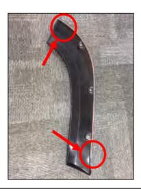
**STEP 22:** Inspect gasket conformity to Fender Flare prior to Installation. Rub gasket if needed, to ensure it is not rolled away from edge. Peel back approximately 2" of the double sided tape liner and fold the liner at 45 degrees to the top leading edge of the Fender Flare.
