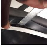
**STEP 21:** Using (4) Mylar Protective Tape strips at the (4) grease pencil marked locations. Install the tape so 50% is on the factory flare and the other 50% can go into the opening made previously by use of the Nylon Pry Tool and fingers to push tape down.
