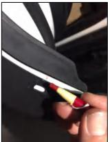
**STEP 19:** While holding Fender Flare onto vehicle, open door to first stop. Ensure Fender Flare is still in position of best fit. Using a grease pencil, mark the center of each slot (4) onto the factory flare. Remove Fender Flare from door.
