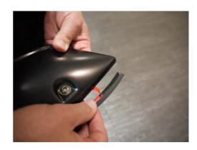
**STEP 2:** Attach the included rubber seal to the Fender Flares. Peel back 2" of the adhesive backing and position on the Fender Flare. Attach the seal to the Fender Flare, peeling back a few inches at a time. Ensure pressure is used to secure rubber seal to Fender Flare edge. Attach rubber seal along all areas the Fender Flare will make contact with the vehicle body. Note: Front and Rear extrusion differs. Rear extrusion will have double sided tape to adhere to both Flare and vehicle.
