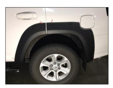
**STEP 25:** Close the door and review how the door piece lines up with the quarter panel piece. If necessary pull slight outward pressure on either flare to disengage the double sided tape from the vehicle and allow the parts to properly align.
