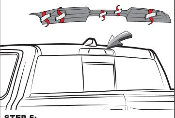
Using the marked position on the masking tape from step 3 as a guide, carefully align the cab spoiler to the roof.
