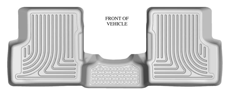
TO EASE INSTALLATION OF YOUR  $2^{\rm nd}$  SEAT JEEP RENEGADE FLOOR LINER, FIRST MOVE THE FRONT SEATS TO THEIR MOST FORWARD POSITIONS. WITH THIS DONE, INSERT LINER IN VEHICLE THEN REPOSITION THE FRONT SEATS AS DESIRED.
