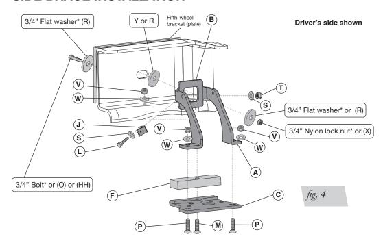
1. Set the upper brace (B) into the driver's and passenger's side frame (Fig. 4).
