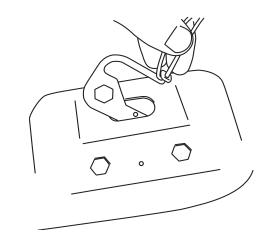
Set rivet nuts into place for alignment. Insert pop rivet through hole in plate and secure in place. Once pop rivet is installed remove string or wire from Reinforcement Plate. NOTE: Verify plate is pulled flush to the body before securing pop rivet.
