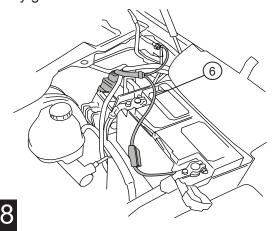
Locate large rubber wire boot on driver side firewall as shown below. Slice small opening as shown below to run trigger wires through.
