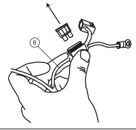
Connect power leads from Controller, Red to positive battery terminal and Black to the vehicle body ground as shown.
