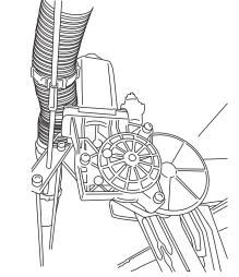
Affix LED light to bracket on rail. Mount front light rearward of front linkage and mount rear light just forward of rear linkage.
