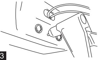
Assemble Hex Bolt (lubricated with soapy water), Washer, Rivet Tool, and Rivet Nut together as shown and place into hex cutouts in sill. An extra Hex Bolt and M8 Washer is supplied to install rivet
