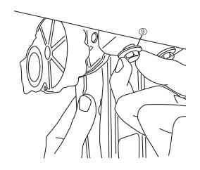
Install provided spacer (22) and M6 bolt (13) into upper mount as shown on both the Drive and Idler linkages. Do not tighten.
