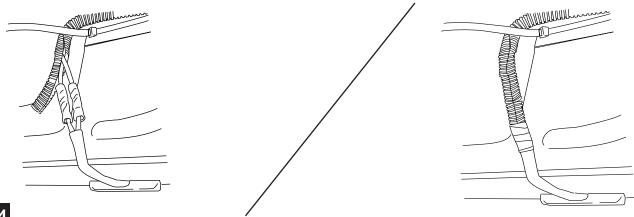
**OBD II install:** Use Supplied Posi Twist connectors to attach the Plug and Play Module to the Harness. Attach matching colors on the harness to the wires on the module. Plug in module to OBD II port on the vehicle. Secure harness with supplied tie wraps.
