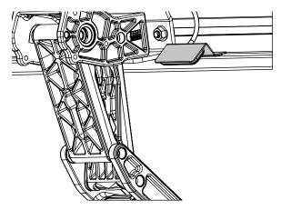
Using supplied butt connectors, connect the lamp wires. Red to Red, Black to Black. Once Crimped use heat gun to shrink tube. Close and wrap conduit with electrical tape. Secure all loose wires with cable ties. Pull lamp wires upward to avoid any wire snagging.
