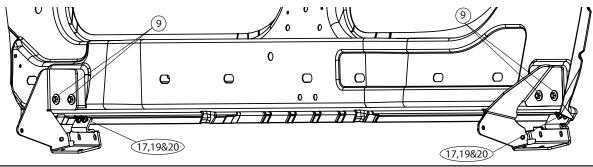
Insert and position Carriage bolts (16) into slot on rail (4). Insert from either end of rail. Using Flange Nuts (17) provided assemble rail to Brackets onto the rail. Next install Flange Bolt (14) and Flange Nut (10) onto bracket tab. Driver side shown. Dimensions shown are for reference. *Torque flange nuts to 16ft-lbs.*
