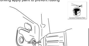
Once hole is drilled insert a piece of string or wire through hole in Reinforcement Plate. Set plate into position.
