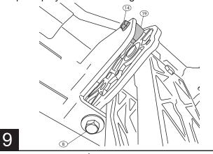
Thread supplied bolts 2x (8) into Front Idler Linkage. Repeat step for Rear Drive Linkage. Do not tighten.
