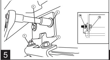
Install provided spacer (19) and M6 bolt (12) into upper mount as shown on both the Drive and Idler linkages. Do not tighten.
