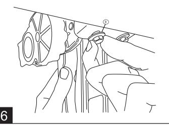
Slide mounting T-nut into position, Center board in rail pocket. Tighten fasteners to 10 ft-lbs.
