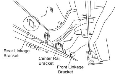
Set Brackets into position and use provided M8 Bolts (21) and washer (15) on outside and provided M8 nuts on the backside. Do not tighten.
