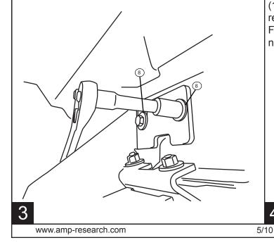
Set Rail up into position. Start with rear bracket work towards the front brackets. Attach Carriage bolts 5x (17) and Flange Nut 5X (18). Center rail at front and rear door line. Torque Flange Nuts to 16 ft-lbs. Insert Flange bolt (13) and nut (18) into side of bracket. Do not tighten.
