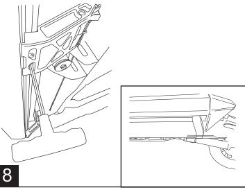
Attach motor to harness. Using a 4mm hex Torque to 36 in-Lbs.
