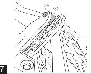
Using a 13mm socket Torque linkage bolts 4x (8) from step 5 to 16 ft-lbs Next use a 10mm socket, torque linkage spacer bolt 2x (12) from step 6 to 8 ft-lbs. Once linkages are tight cycle board to verify steps deploy under own weight.
