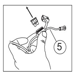
Attach wire harness to controller (make sure connector locking tabs fully engage). Mount controller with the two 11" tie wraps to factory conduit.
